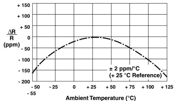
**Note:** The TCR values for  $< 80 \Omega$  are influenced by the termination composition and the result in deviation from this curve
