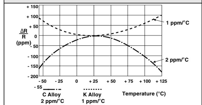
Vishay Foil Resistors High Precision Foil Resistor with TCR of  $\pm 2.0 \text{ ppm}/^\circ\text{C}$ ,
