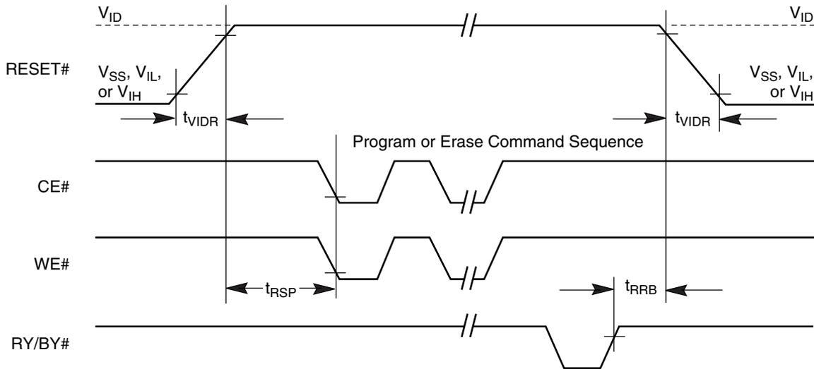
Figure 23. Temporary Sector Group Unprotect Timing Diagram
