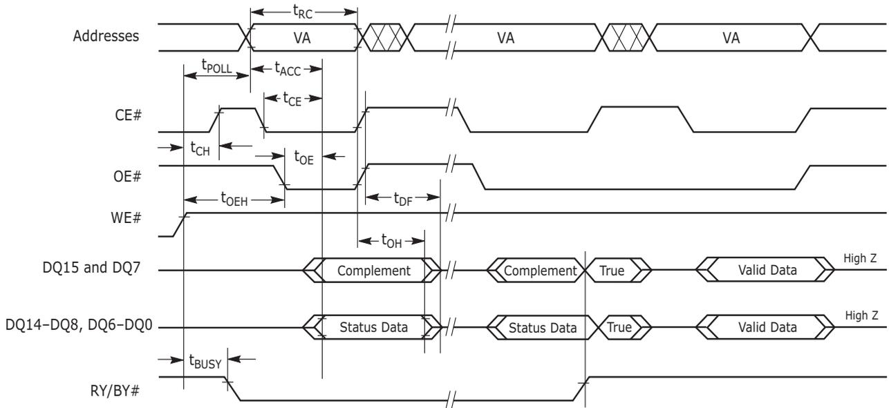
**Note:** VA = Valid address. Illustration shows first status cycle after command sequence, last status read cycle, and array data read cycle.
