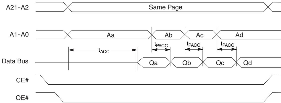
\* Figure shows device in word mode. Addresses are A1–A-1 for byte mode.
