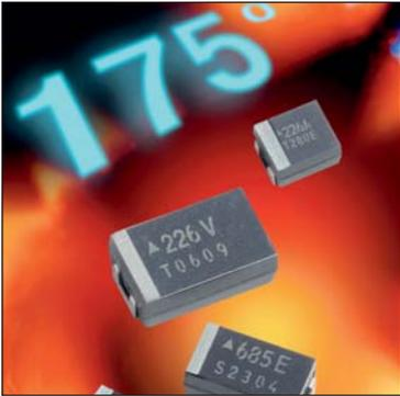
The THJ surface mount series combines high temperature operation and higher basic reliability for optimal performance in high temperature automotive and industry applications. The operational temperature is up to +175°C with 50% voltage derating. The level of reliability of this tantalum product is 0.5% / 1000 hours at rated voltage,
