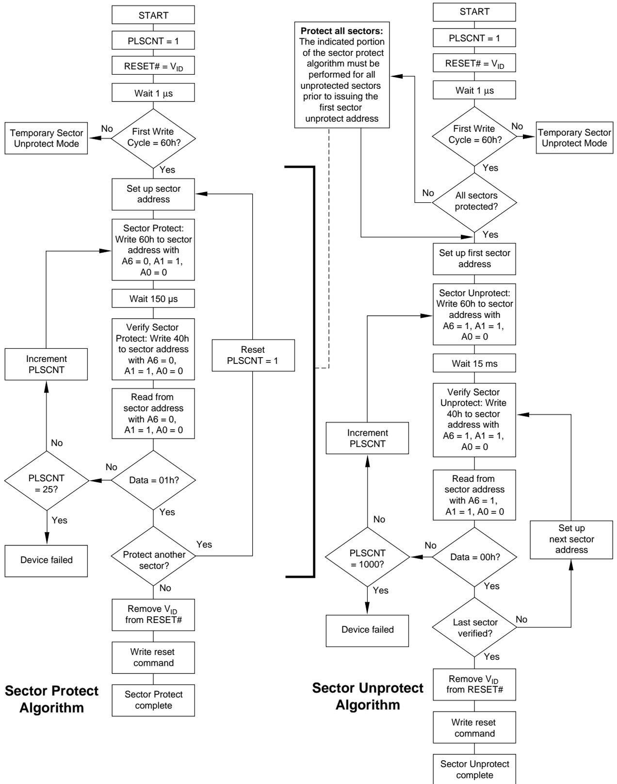
Figure 2. In-System Sector Protect/ Sector Unprotect Algorithms
