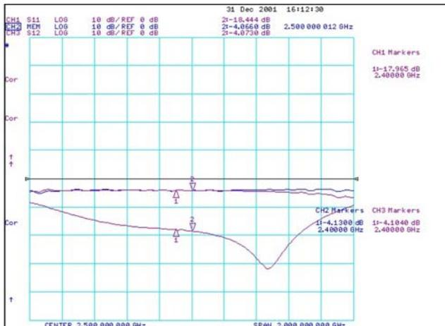
Note: -4.1dB should include 0.4dB microstrip line loss
