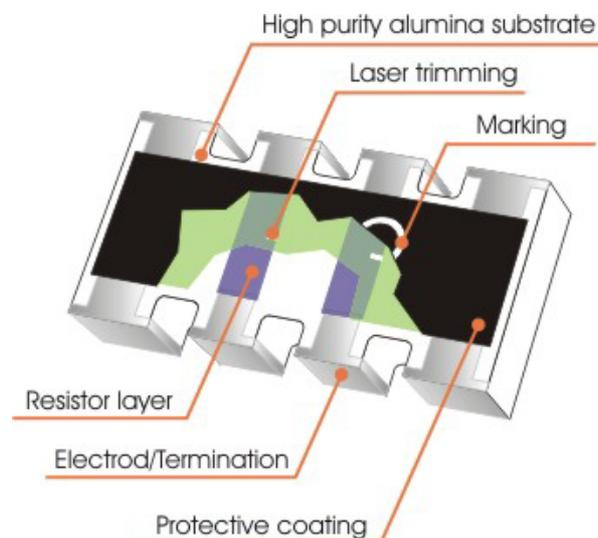
Fig 1. Construction of a Chip-R array WA06X, 5% product
