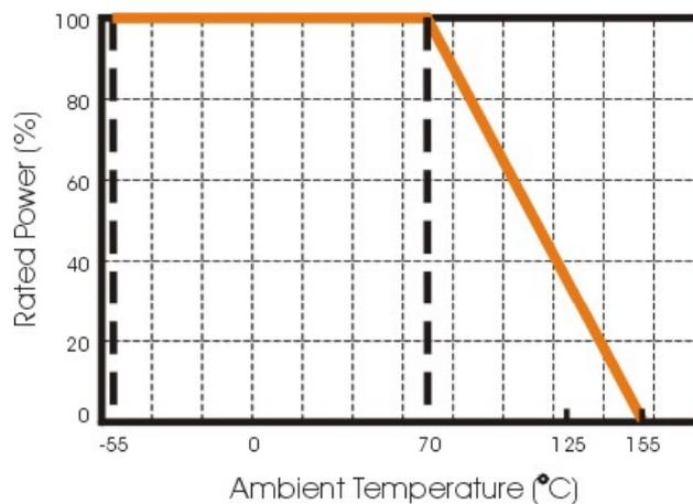
Figure 2. Maximum dissipation in percentage of rated power
