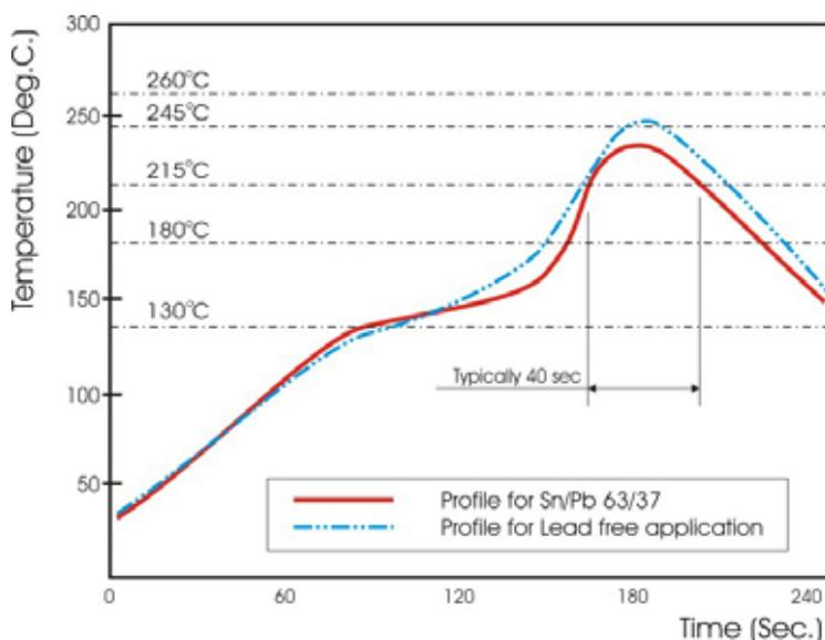
Fig 3. Infrared soldering profile for Chip Resistors array
