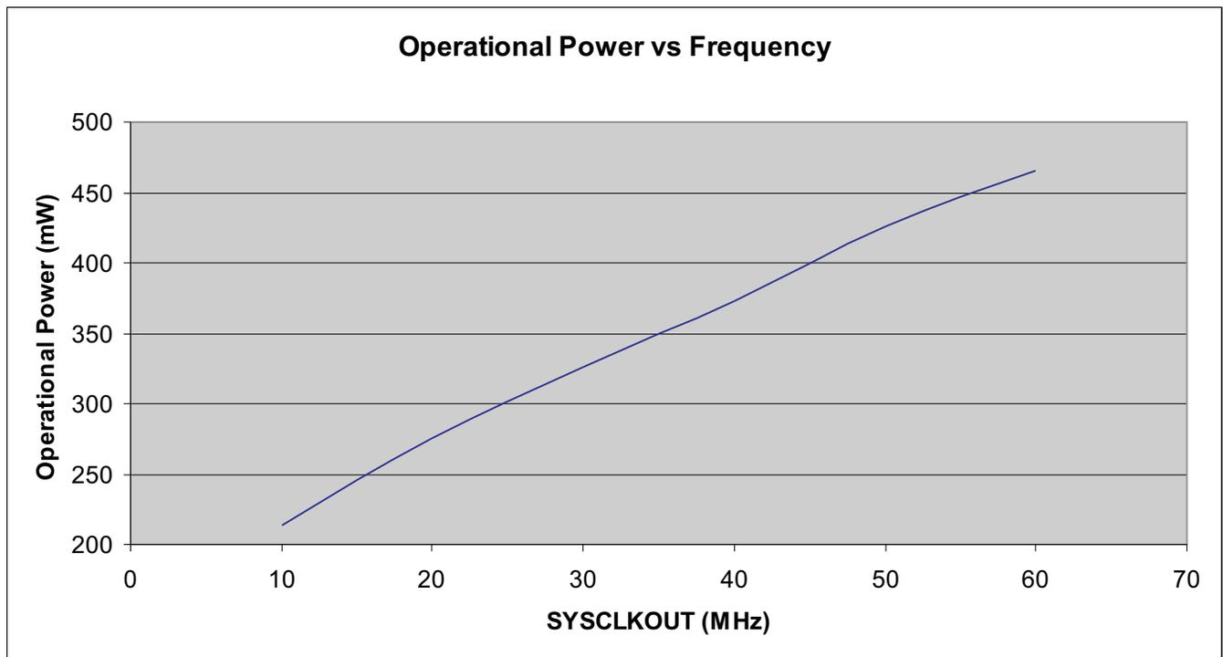
Figure 6-2. Typical Operational Power Versus Frequency (F2803x)
