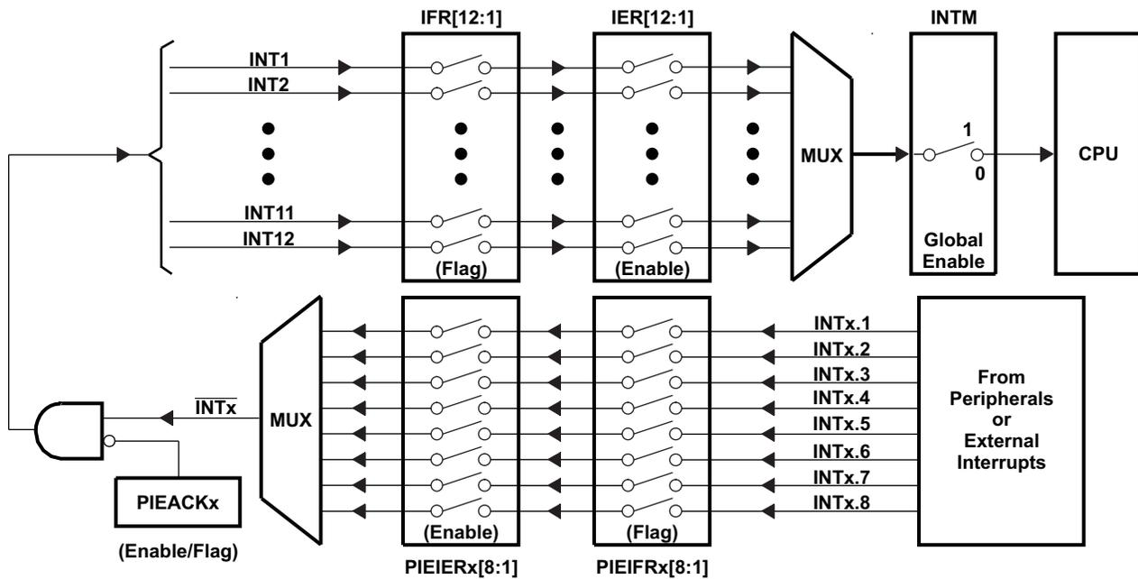
Figure 3-6. Multiplexing of Interrupts Using the PIE Block
