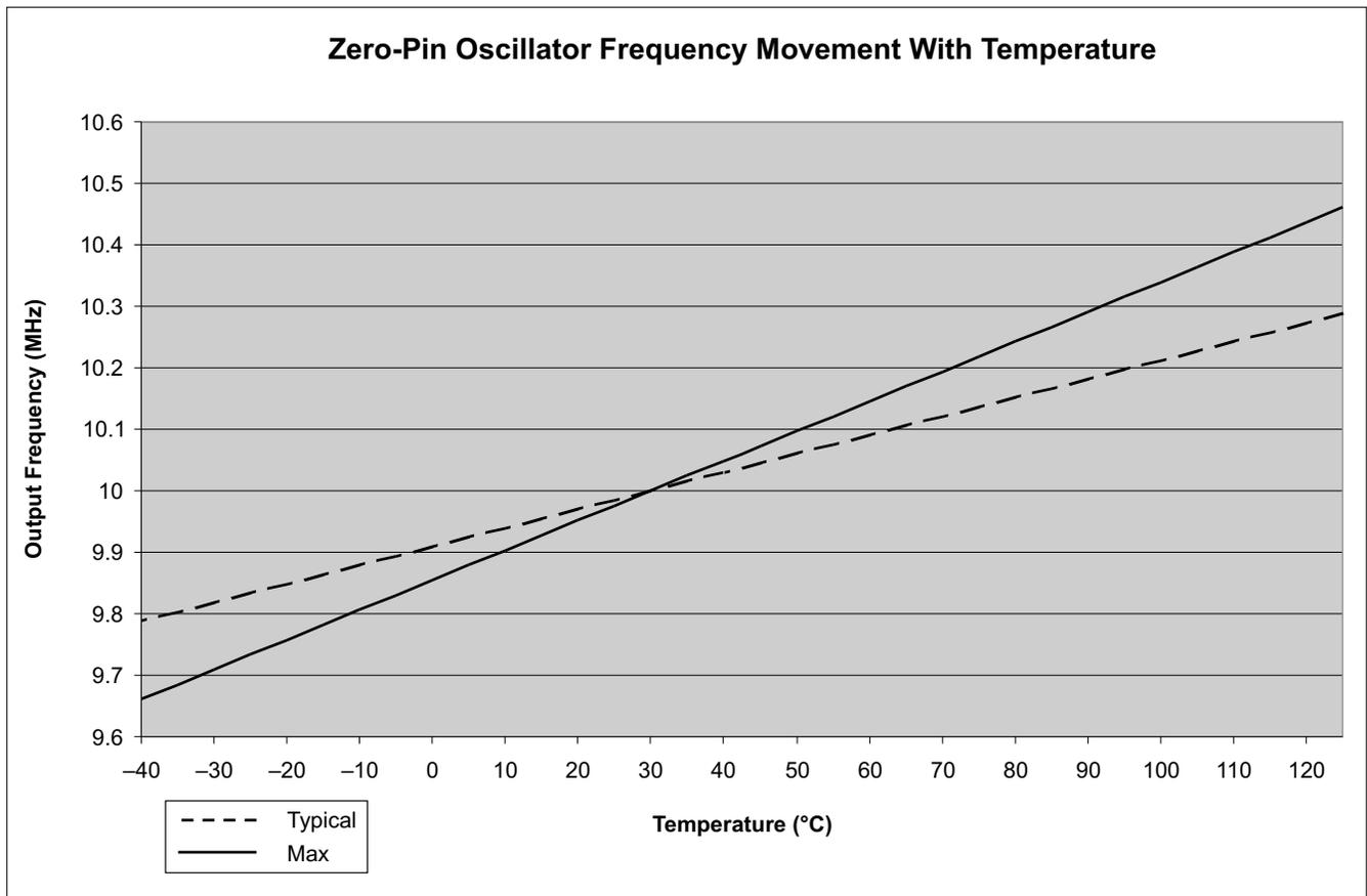
**Figure 6-6. Zero-Pin Oscillator Frequency Movement With Temperature**
