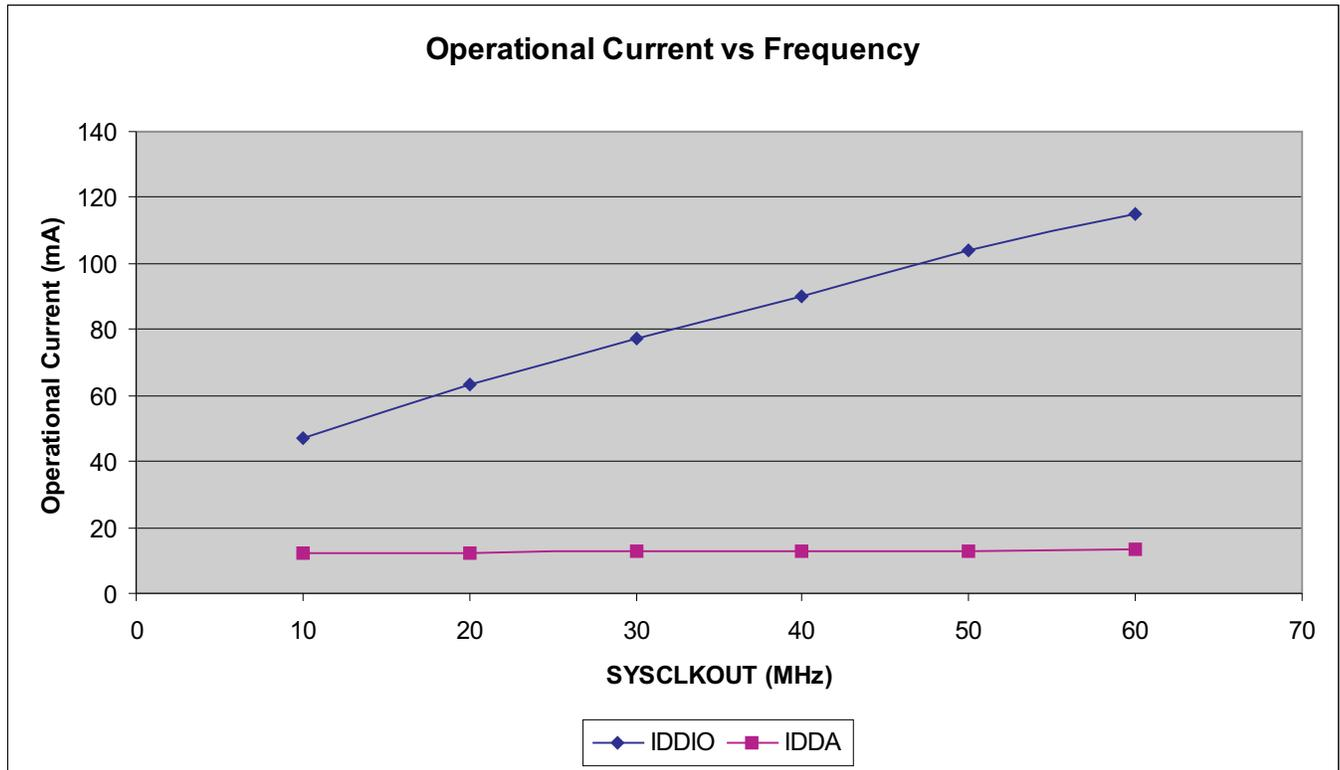
Figure 6-1. Typical Operational Current Versus Frequency (F2803x)
