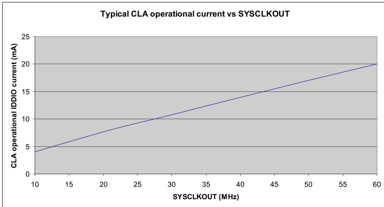
Figure 6-3. Typical CLA Operational Current Versus SYSCLKOUT
