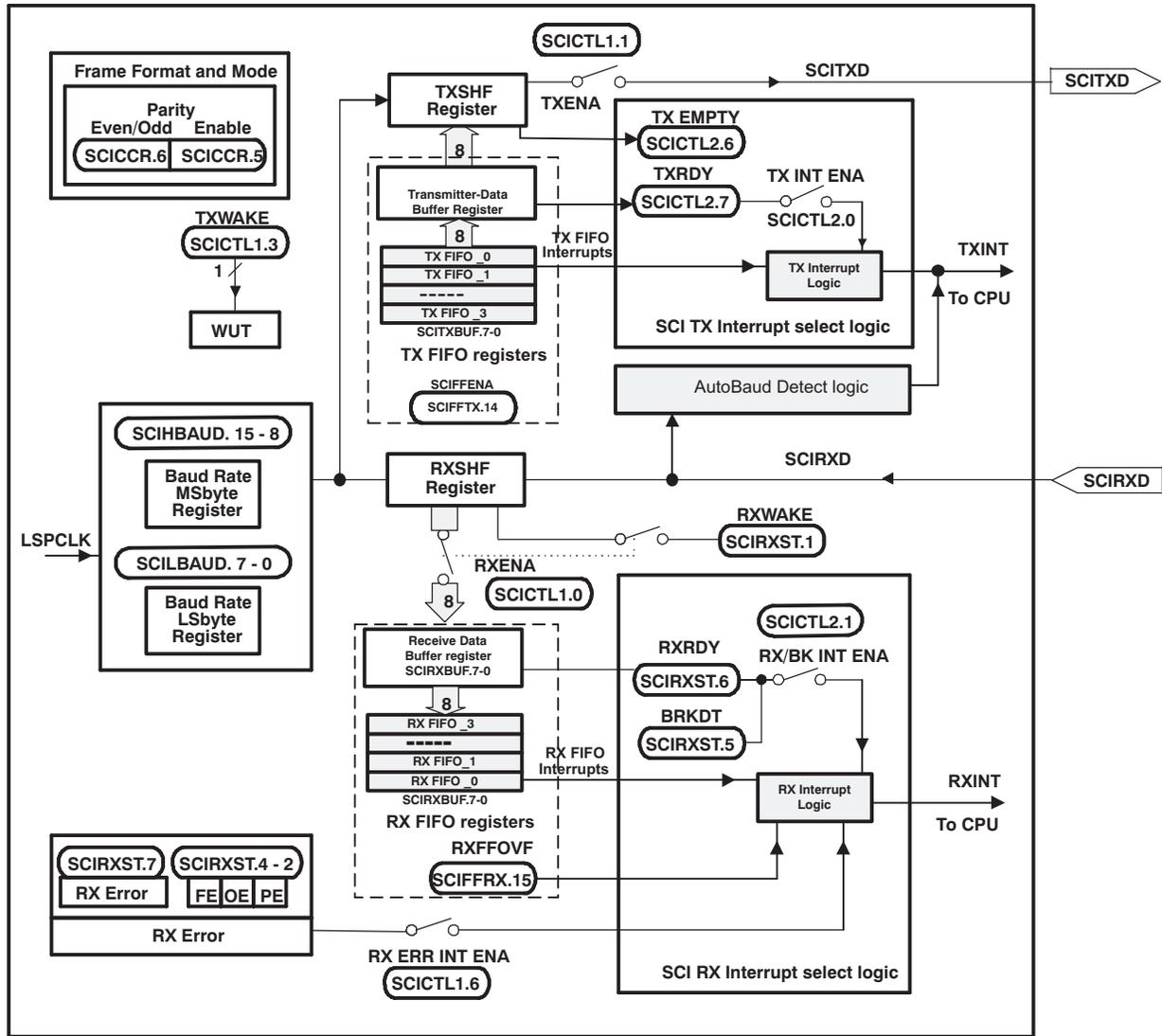
Figure 4-7. Serial Communications Interface (SCI) Module Block Diagram
