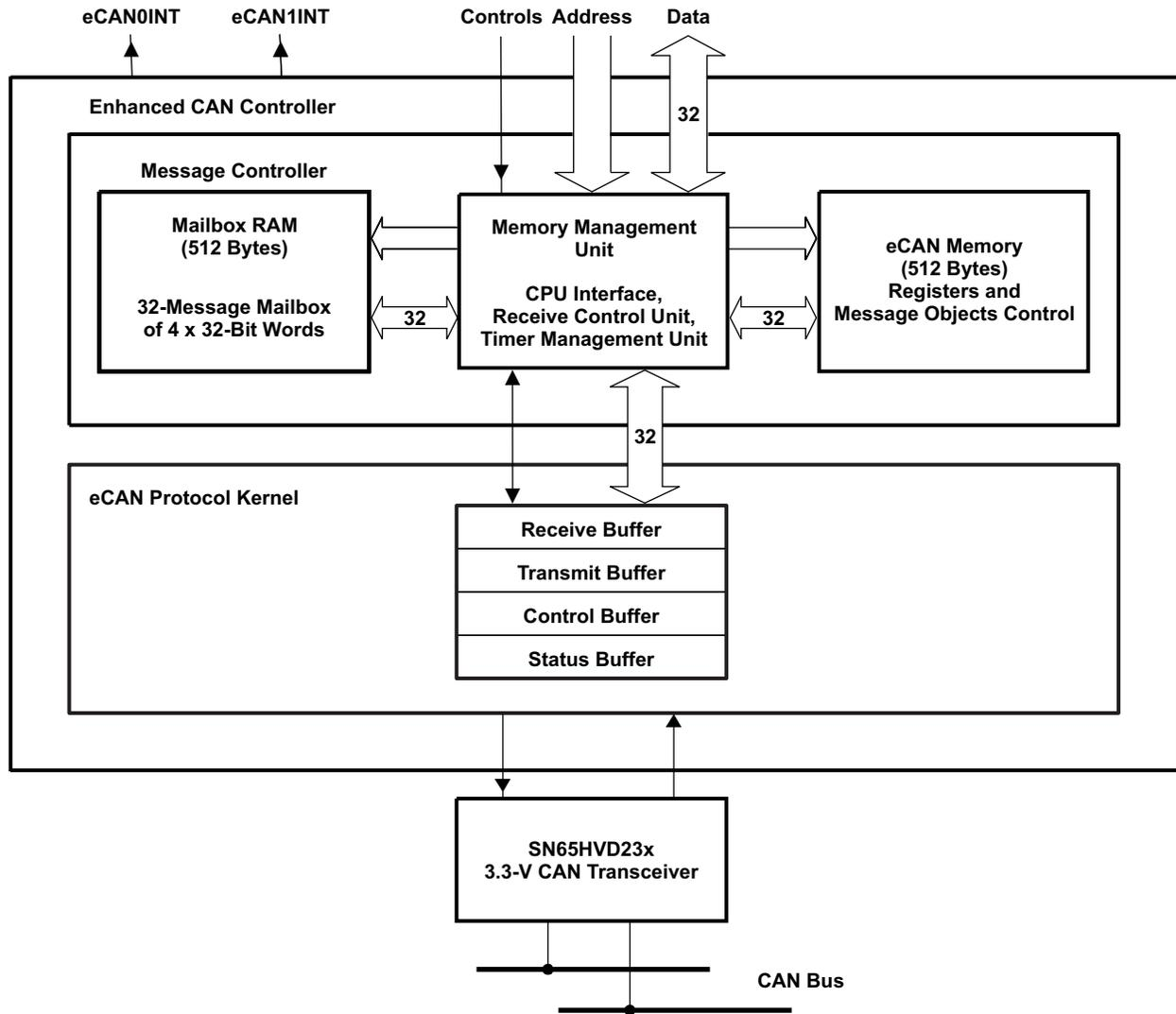
Figure 4-9. eCAN Block Diagram and Interface Circuit
