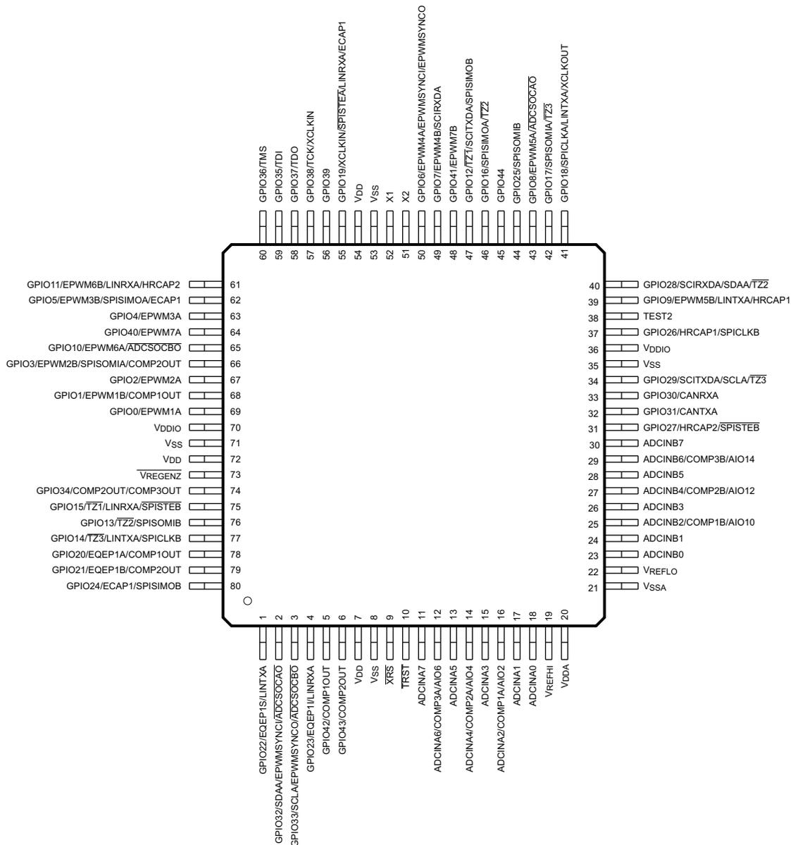
Figure 2-3. 2803x 80-Pin PN LQFP (Top View)
