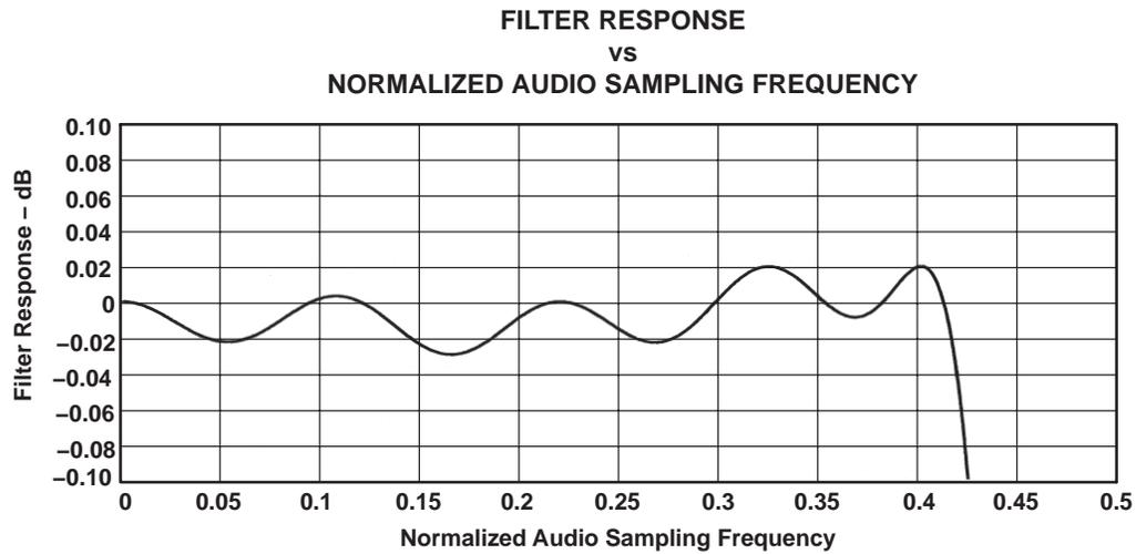
**Figure 3–22. DAC Digital Filter Ripple 1: USB Mode Only**
