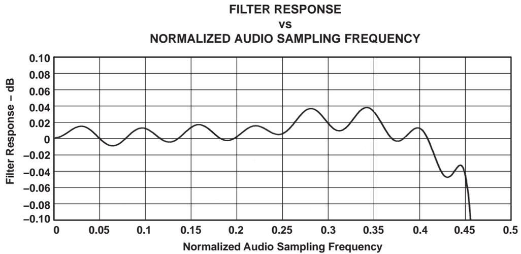
**Figure 3–20. DAC Digital Filter Ripple 0: USB Mode**
