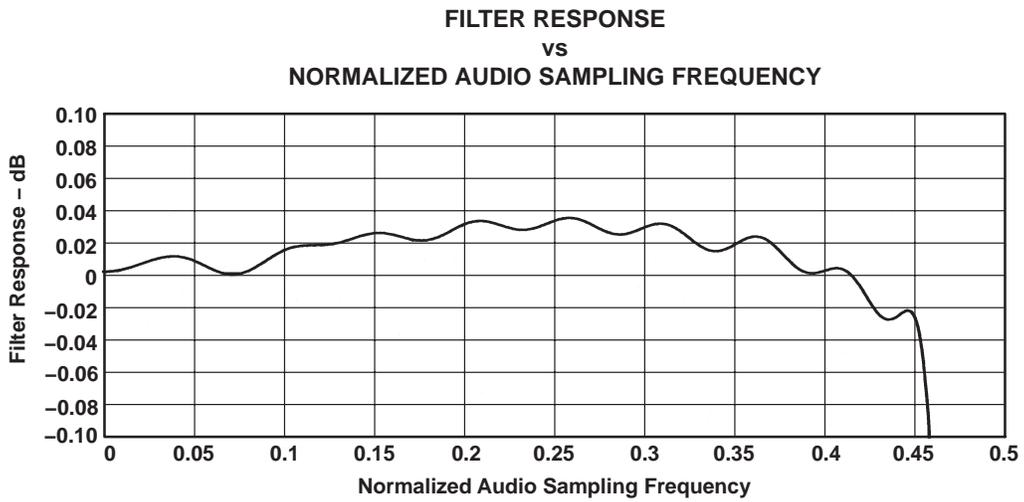
**Figure 3–12. ADC Digital Filter Ripple 0: USB
