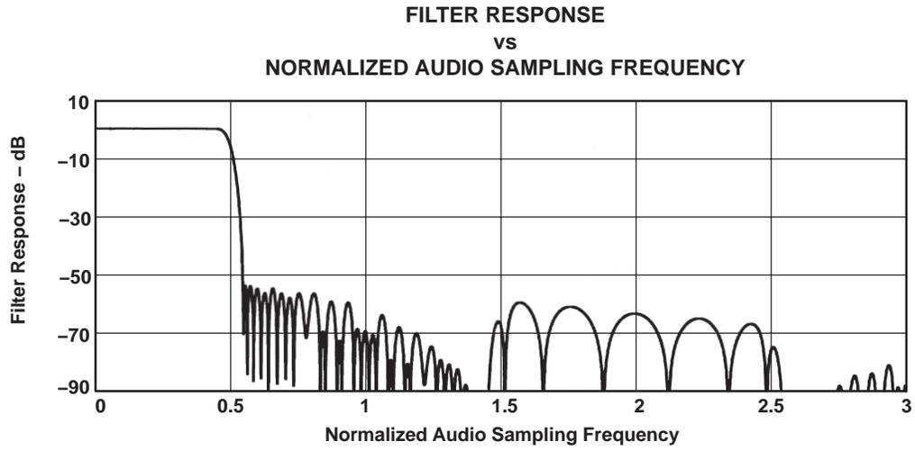
**Figure 3–19. DAC Digital Filter Response 0: USB Mode**
