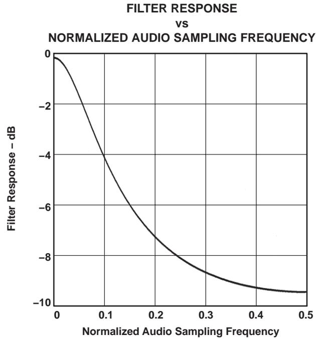
**Figure 3-9. Digital De-Emphasis Filter Response – 44.1 kHz Sampling**
