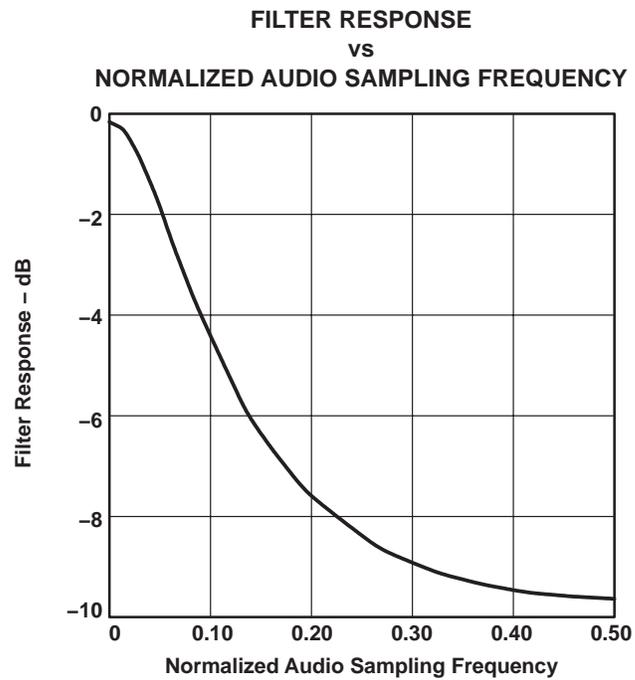
**Figure 3-10. Digital De-Emphasis Filter Response – 48 kHz Sampling**
