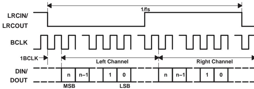
Figure 3-7. I<sup>2</sup>S Mode Timing
