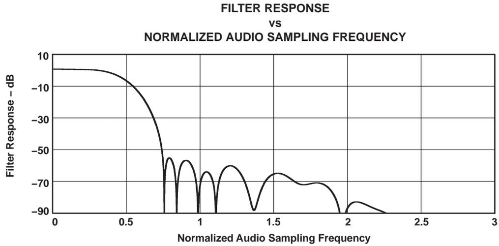
**Figure 3–25. DAC Digital Filter Response 3: USB Mode Only**
