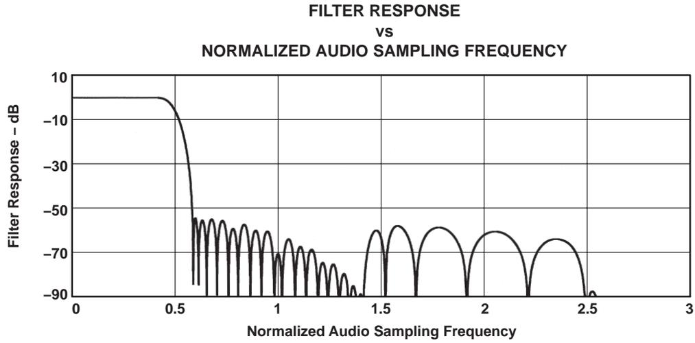
**Figure 3–21. DAC Digital Filter Response 1: USB Mode Only**
