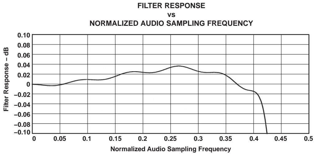
**Figure 3–14. ADC Digital Filter Ripple 1: USB Mode Only**
