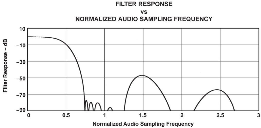
**Figure 3-15. ADC Digital Filter Response 2: USB mode and Normal Modes
