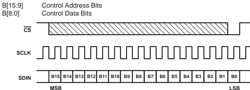
Figure 3–1. SPI Timing
