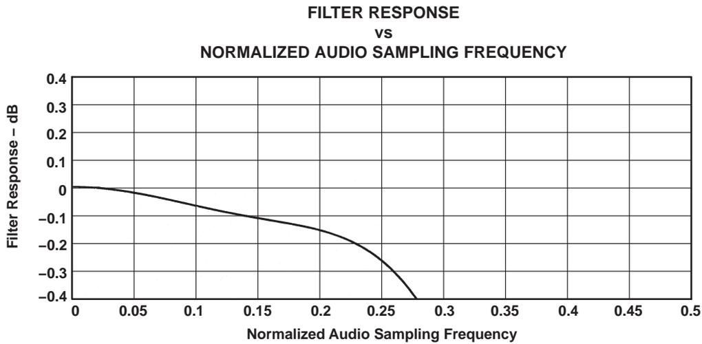
**Figure 3–26. DAC Digital Filter Ripple 3: USB Mode Only**
