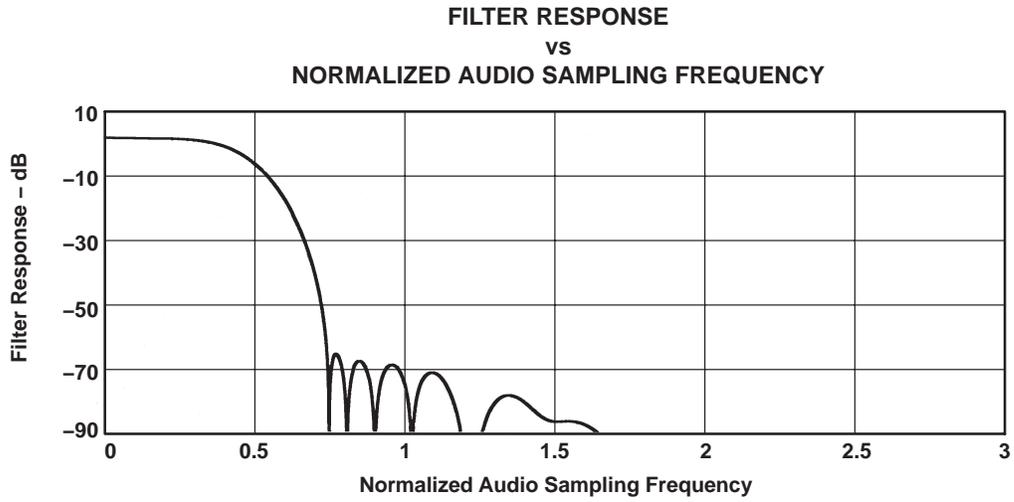
**Figure 3-17. ADC Digital Filter Response 3: USB Mode Only**
