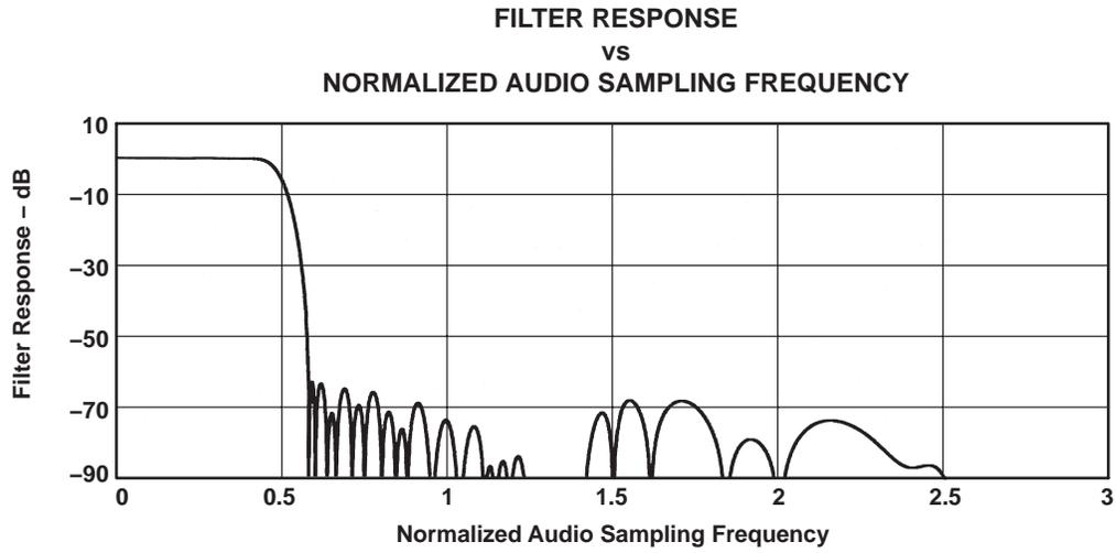
**Figure 3–13. ADC Digital Filter Response 1: USB Mode Only**
