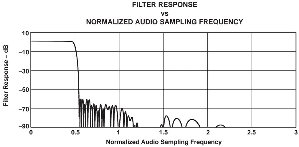
**Figure 3–11. ADC Digital Filter Response 0: USB Mode
