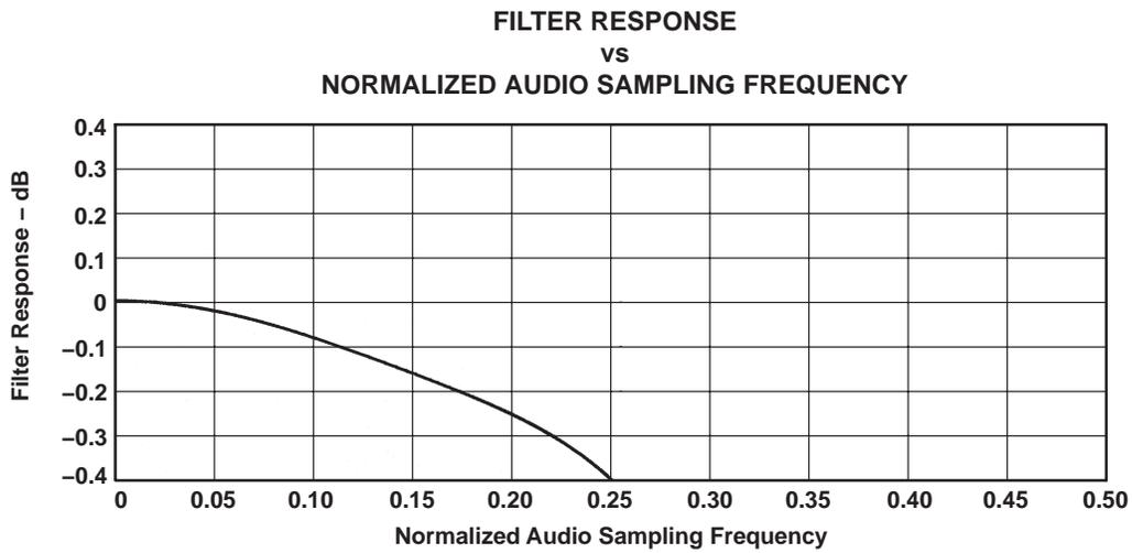
**Figure 3-18. ADC Digital Filter Ripple 3: USB Mode Only**
