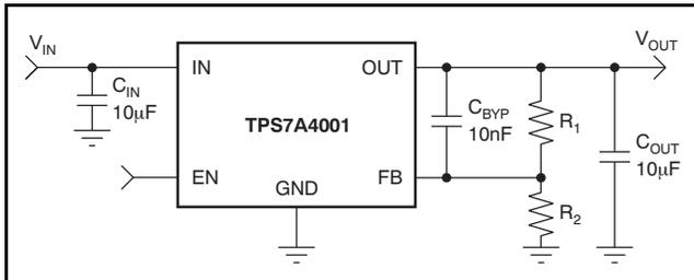
**Figure 13. Adjustable Operation for Maximum AC Performance**
