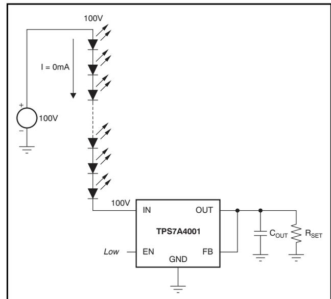
Figure 15. LED Array Driver with Regulator Disabled
