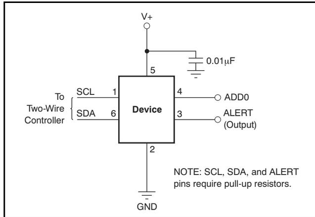
Figure 7. Typical Connections
