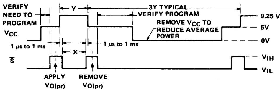
**FIGURE 2 – VOLTAGE WAVEFORMS FOR PROGRAMMING**
