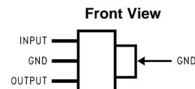
**Figure 2. SOT-223 Plastic Package**
