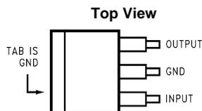
**Figure 3. DPAK/TO-263 Surface-Mount Package**
