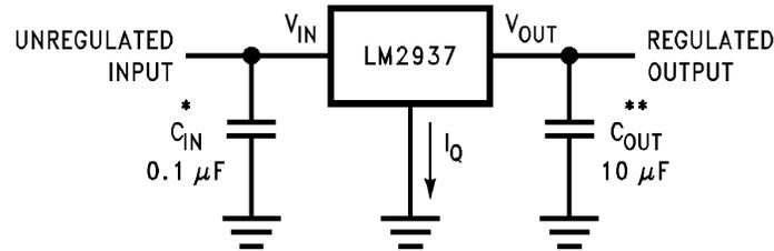
\* Required if the regulator is located more than 3 inches from the power supply filter capacitors.
