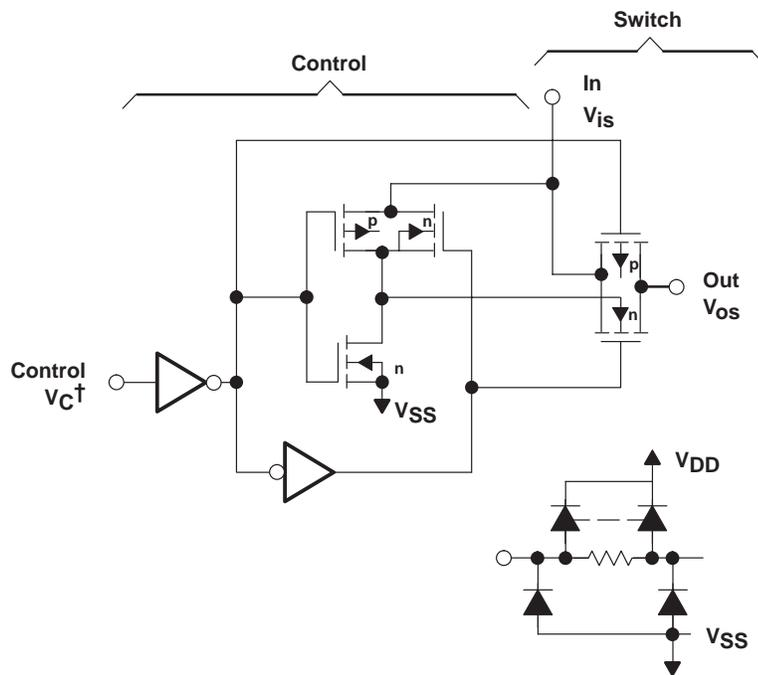
† All control inputs are protected by the CMOS protection network.
