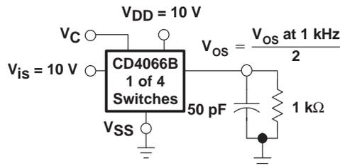
All unused terminals are connected to  $V_{SS}$ .
