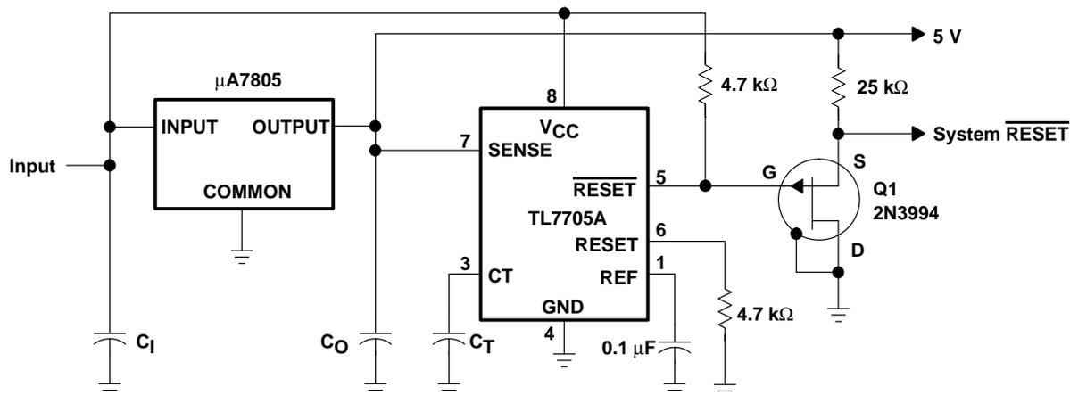
Figure 8. Eliminating Undefined States Using a P-Channel JFET
