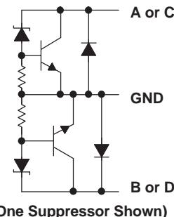
NOTE: All GND terminals should be connected to ground.
