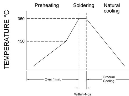
Figure 2. Iron Soldering
