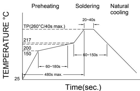
Figure 1. Re-flow Soldering
