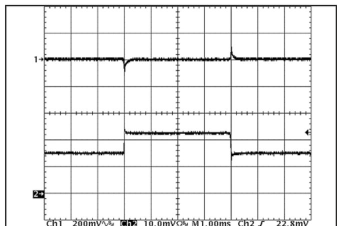
Figure 12: Output voltage response to step-change in load current (50%-75%-50% of I<sub>out</sub>(max); dI/dt = 5A/μs). Load cap: 480μF, 15 mΩ ESR tantalum cap and 1μF ceramic cap. Top trace: V<sub>out</sub> (200mV/div), Bottom trace: I<sub>out</sub> (20A/div).
