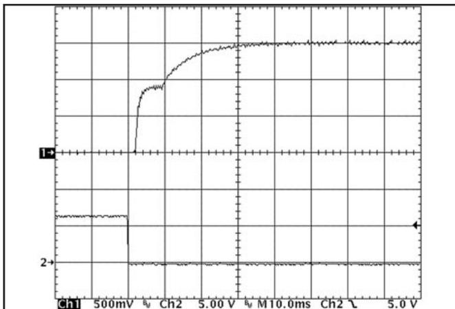
Figure 9: Turn-on transient at full load (resistive load) (10 ms/div). Input voltage pre-applied. Top Trace: V<sub>out</sub> (0.5V/div). Bottom Trace: ON/OFF input (5V/div).
