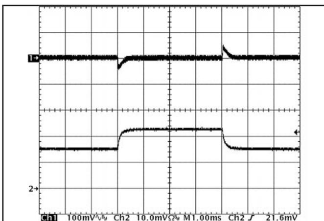
Figure 11: Output voltage response to step-change in load current (50%-75%-50% of I<sub>out</sub>(max); dI/dt = 0.1A/μs). Load cap: 15μF, 450 mΩ ESR tantalum cap and 1μF ceramic cap. Top trace: V<sub>out</sub> (100mV/div), Bottom trace: I<sub>out</sub> (20A/div).
