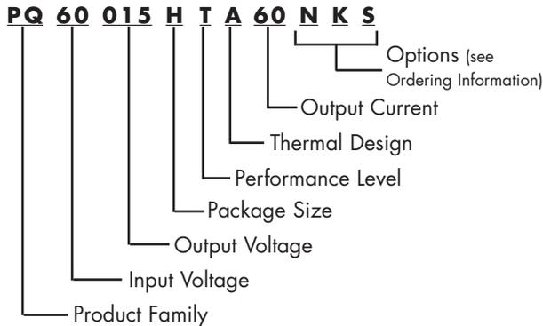
The first 12 characters comprise the base part number and the last 3 characters indicate available options. Although there are no default values for enable logic and pin length, the most common options are negative logic and 0.145" pins. These part numbers are more likely to be readily available in stock for evaluation and prototype quantities.
