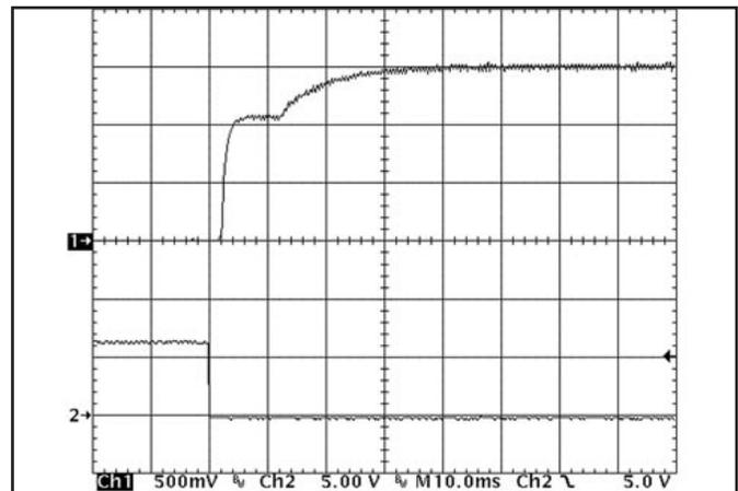
Figure 10: Turn-on transient at zero load (10 ms/div). Top Trace: V<sub>out</sub> (0.5V/div). Bottom Trace: ON/OFF input (5V/div).
