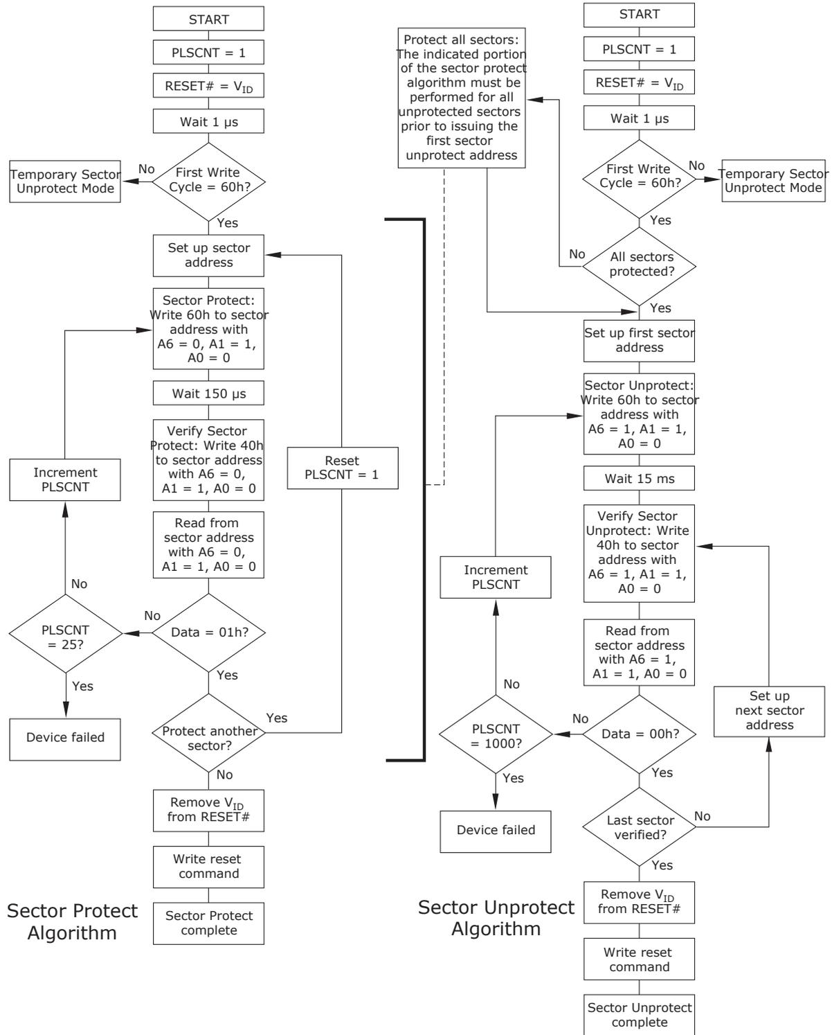
Figure 2. In-System Sector Protect/Sector Unprotect Algorithms
