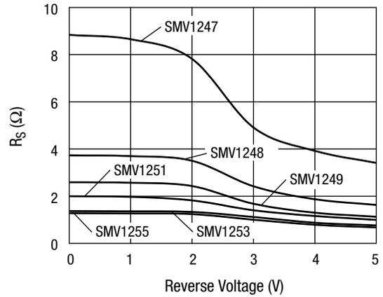
**Series Resistance vs. Reverse Voltage @ 500 MHz**
