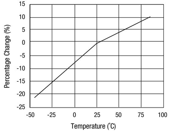
**Relative Series Resistance Change vs. Temperature @ 500 MHz**
