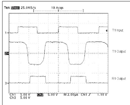
Figure 14. SP3220EU Driver Loopback Test Results at 1Mb/s
