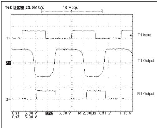
Figure 13. SP3220EB Driver Loopback Test Results at 250Kbps
