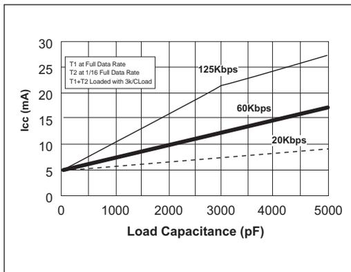
Figure 1.  $I_{CC}$  vs Load Capacitance for the SP3220EB.
