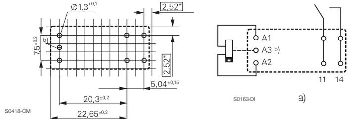
\*) With the recommended PCB hole sizes a grid pattern from 2.5mm to 2.54mm can be used.
