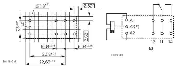
\*) With the recommended PCB hole sizes a grid pattern from 2.5mm to 2.54mm can be used.
