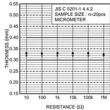
Fig.4 Dimensions (thickness)
