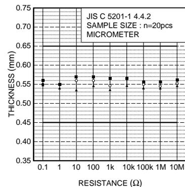
Fig.4 Dimensions (thickness)
