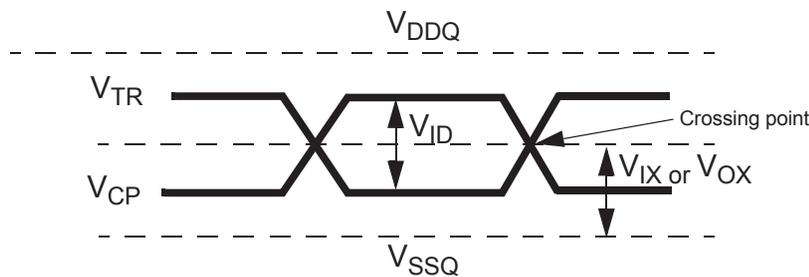
NOTE 1 VID(AC) specifies the input differential voltage  $|V_{TR} - V_{CP}|$  required for switching, where  $V_{TR}$  is the true input signal (such as CK, DQS, LDQS or UDQS) and  $V_{CP}$  is the complementary input signal (such as  $\overline{CK}$ ,  $\overline{DQS}$ ,  $\overline{LDQS}$  or  $\overline{UDQS}$ ). The minimum value is equal to  $V_{IH(AC)} - V_{IL(AC)}$ .
