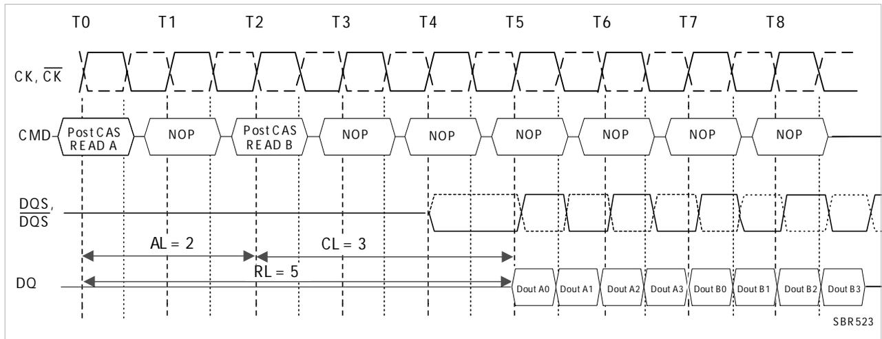
The seamless burst read operation is supported by enabling a read command at every BL / 2 number of clocks. This operation is allowed regardless of same or different banks as long as the banks are activated.
