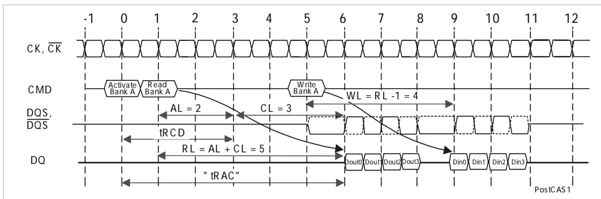
**Read followed by a write to the same bank, Activate to Read delay <  $t_{\text{RCDmin}}$ :**
