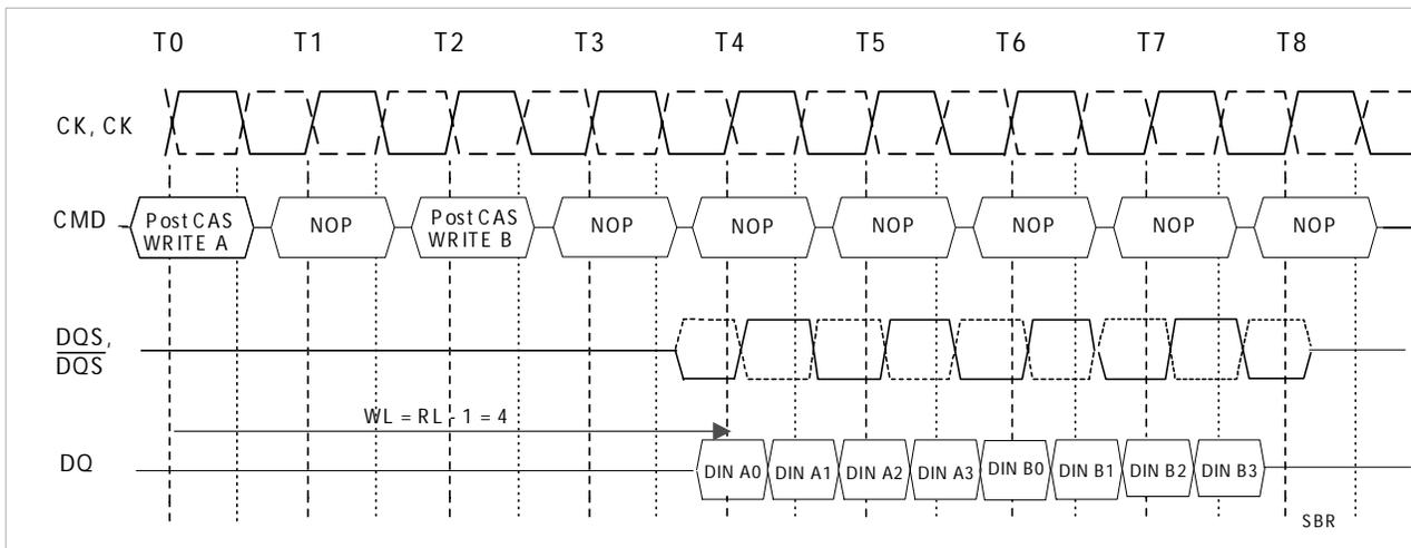
The seamless burst write operation is supported by enabling a write command every  $BL / 2$  number of clocks. This operation is allowed regardless of same or different banks as long as the banks are activated.
