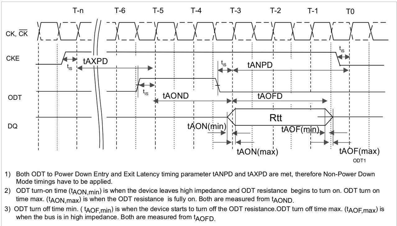
ODT Timing for Precharge Power-Down and Low Power Power-Down Mode
