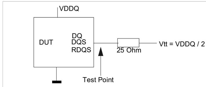
Output slew rate for falling and rising edges is measured between  $V_{TT} - 250\text{ mV}$  and  $V_{TT} + 250\text{ mV}$  for single ended signals. For differential signals (e.g.  $DQS - \overline{DQS}$ ) output slew rate is measured between  $DQS - \overline{DQS} = -500\text{ mV}$  and  $DQS - \overline{DQS} = +500\text{ mV}$ . Output slew rate is guaranteed by design, but is not necessarily tested on each device.
