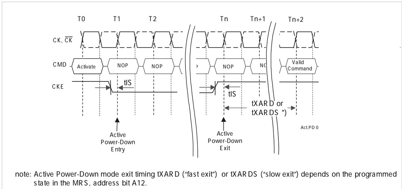
Active Power-Down Mode Entry and Exit after a Read Burst: RL = 4 (AL = 1, CL = 3), BL = 4
