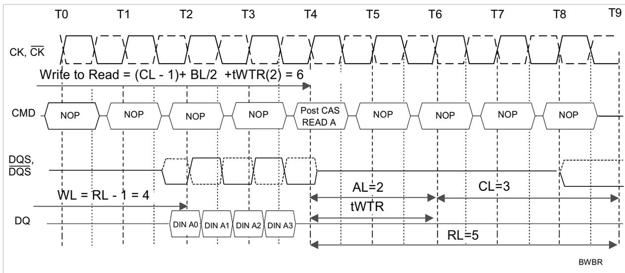
The minimum number of clocks from the burst write command to the burst read command is
