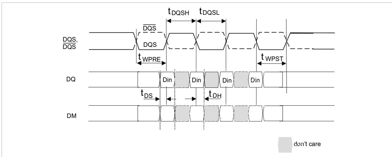
**Burst Write Operation with Data Mask : RL = 3 (AL = 0, CL = 3), WL = 2, tWR = 3 , BL = 4**
