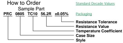
Add "T" at the end of the Case Size portion of the part number for lead free termination.
