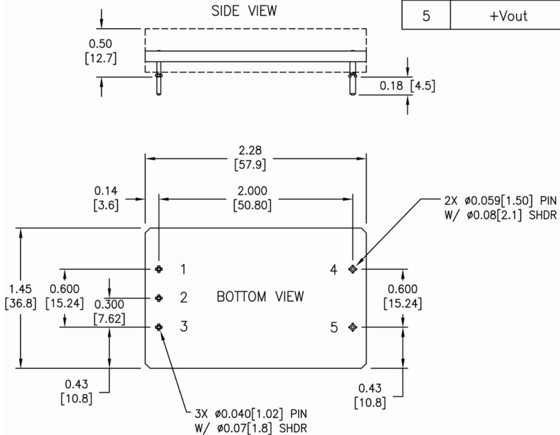
PIN DIAMETER TOLERANCE:  $\pm 0.002$  [0.05]
