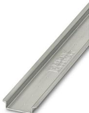
DIN rail, unperforated, acc. to EN 60715, material: Steel, galvanized, passivated with a thick layer, Standard profile, color: silver, Pack of 25 (50 m)
