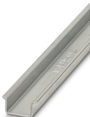
DIN rail, unperforated, acc. to EN 60715, material: Steel, galvanized, passivated with a thick layer, Standard profile 2.3 mm, color: silver, Pack of 10 (20 m)
