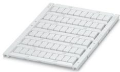
Marker for terminal blocks, Sheet, white, unlabeled, can be labeled with: TOPMARK NEO, TOPMARK LASER, BLUEMARK ID COLOR, BLUEMARK ID, BLUEMARK CLED, THERMOMARK PRIME, THERMOMARK CARD 2.0, THERMOMARK CARD, mounting type: snap in, for terminal block width: 6.2 mm, lettering field size: 5.6 x 10.5 mm, Number of individual labels: 60
