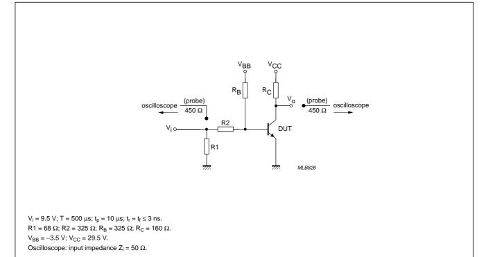
Fig.2 Test circuit for switching times.
