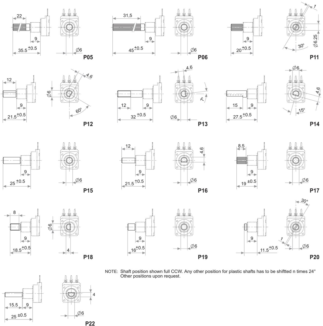
NOTE: Shaft position shown full CCW. Any other position for plastic shafts has to be shifted n times  $24^\circ$ . Other positions upon request.
