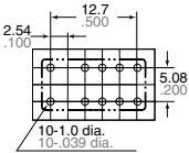
Tolerance:  $\pm 0.1 \pm .004$ **2 coil latching type (L2, LT)**
