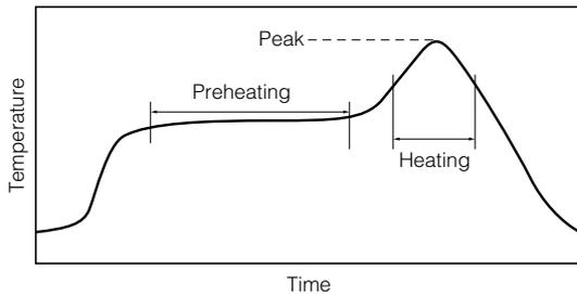
For soldering (Example : Sn/Pb)
