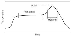
For soldering (Example: Sn/Pb)
