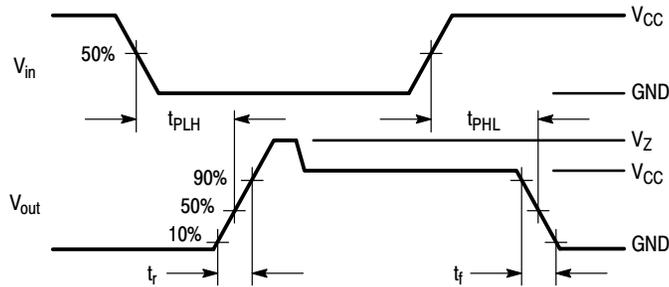
Figure 1. Switching Waveforms
