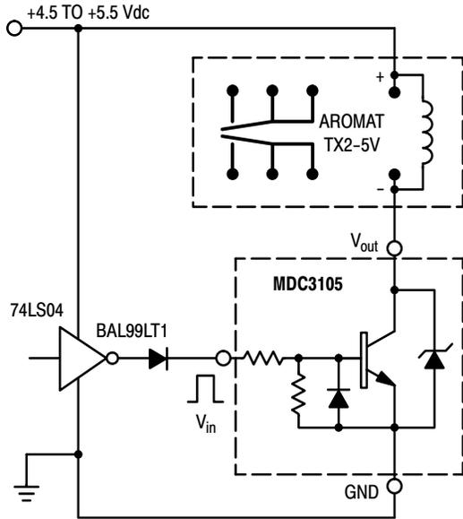
Figure 14. A 140 mW, 5.0 V Relay with TTL Interface
