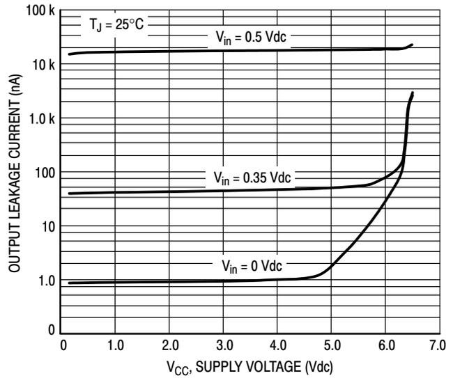
Figure 9. Output Leakage Current versus Supply Voltage
