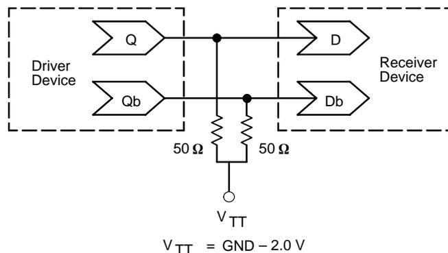
**Figure 1. Typical Termination for Output Driver and Device Evaluation
