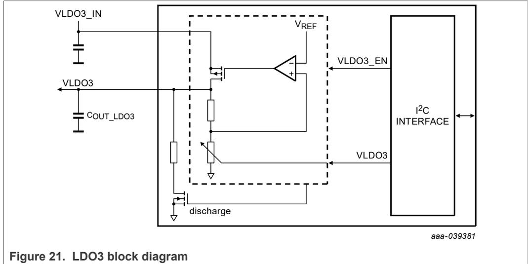
Figure 21. LDO3 block diagram
