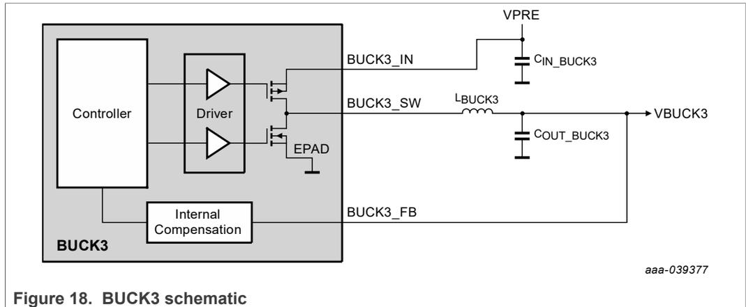
Figure 18. BUCK3 schematic
