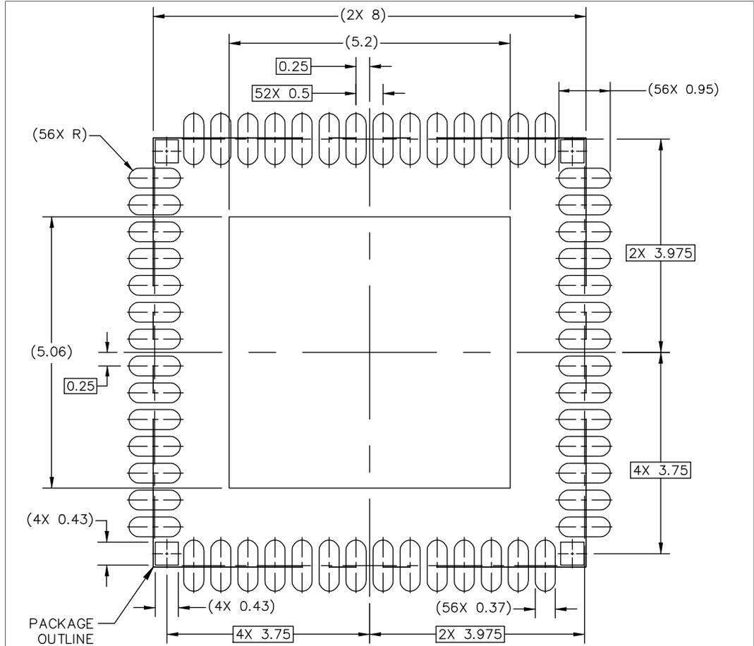
PCB DESIGN GUIDELINES – SOLDER MASK OPENING PATTERN
