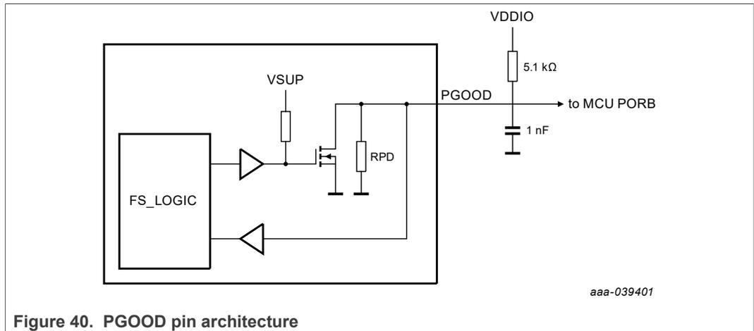
Figure 40. PGOOD pin architecture
