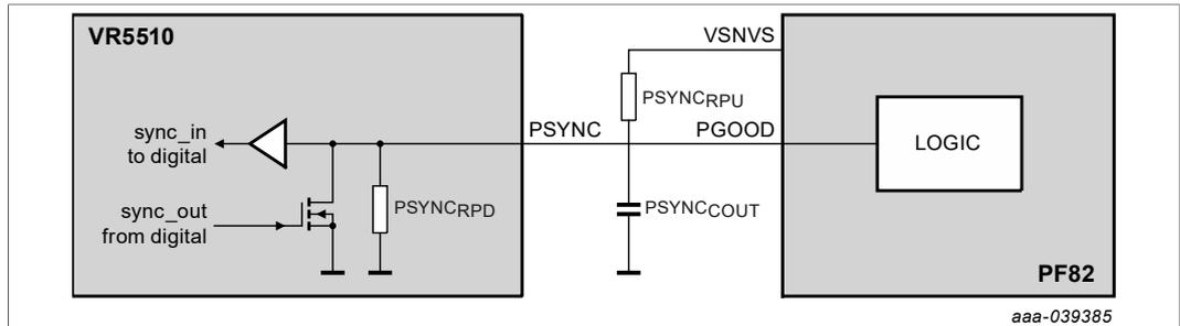
Figure 26. Synchronization of one VR5510 and one PF82
