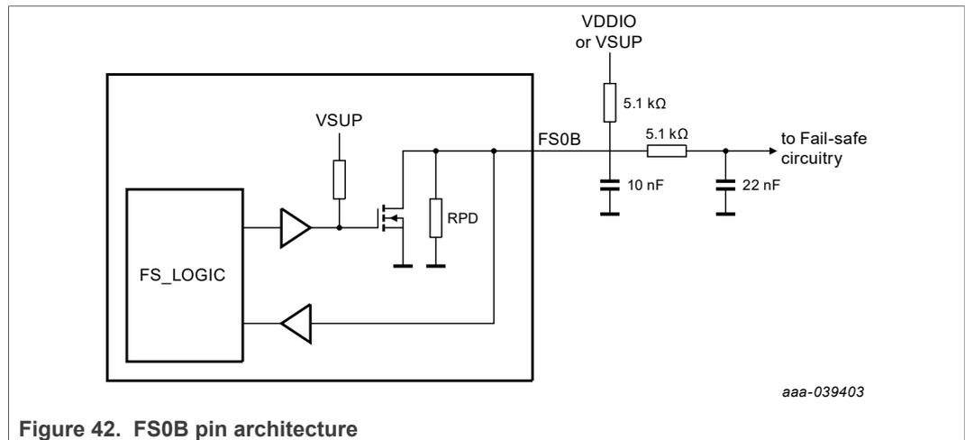
Figure 42. FS0B pin architecture
