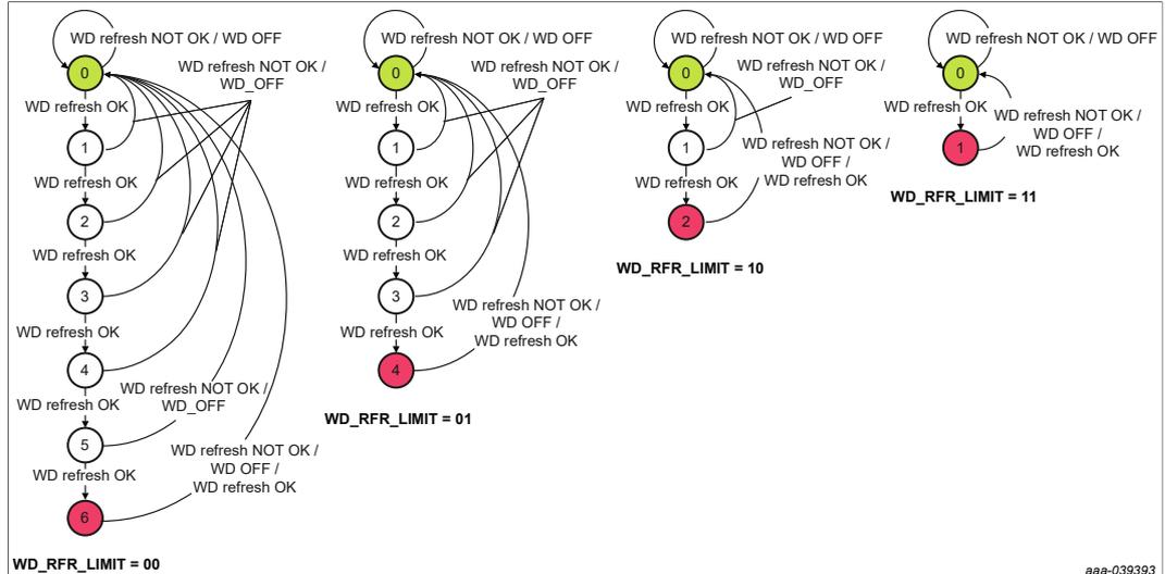
Figure 32. Watchdog refresh counter configurations
