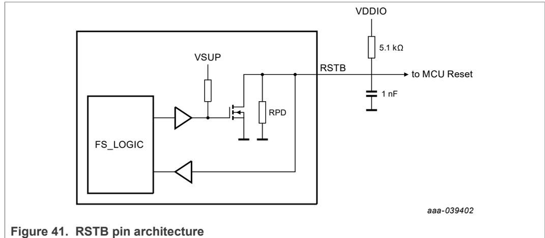
Figure 41. RSTB pin architecture
