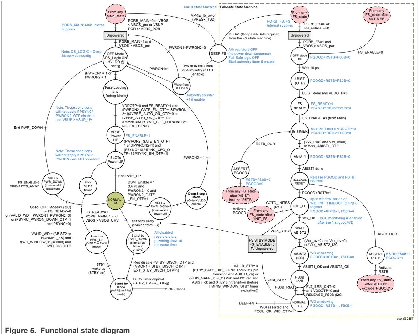
Figure 5. Functional state diagram
