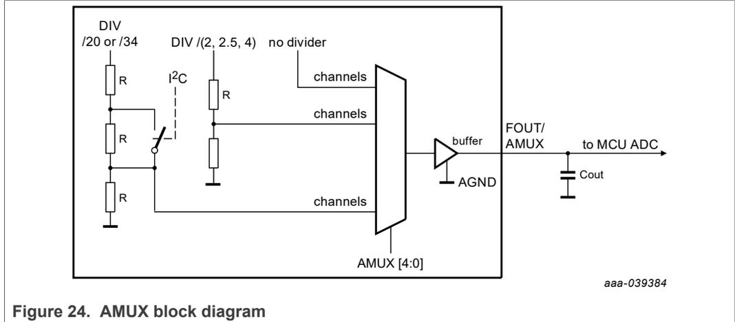
Figure 24. AMUX block diagram
