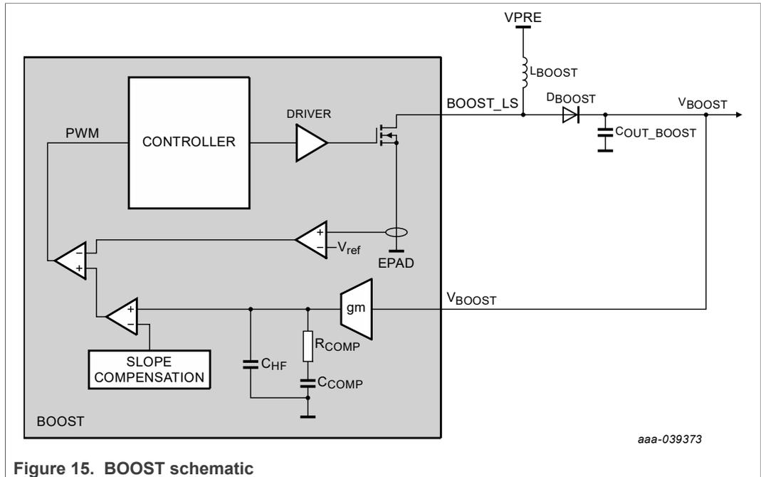
Figure 15. BOOST schematic
