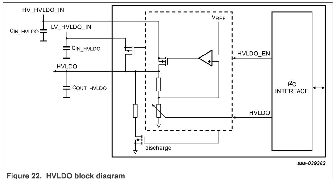
Figure 22. HVLDO block diagram
