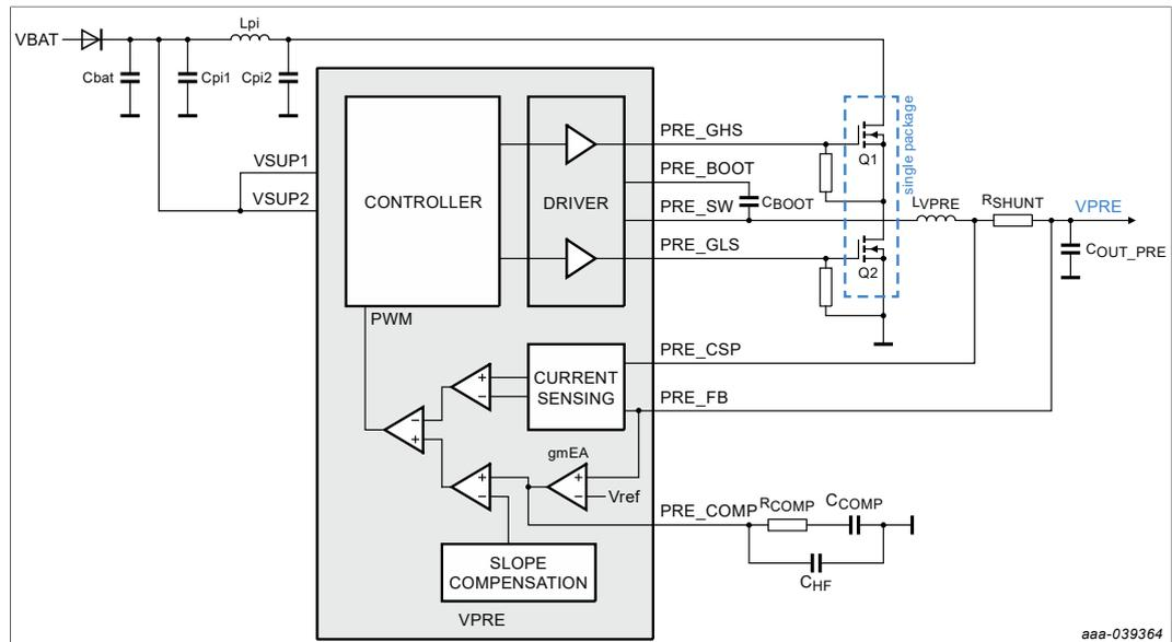
Figure 12. VPRE schematic
