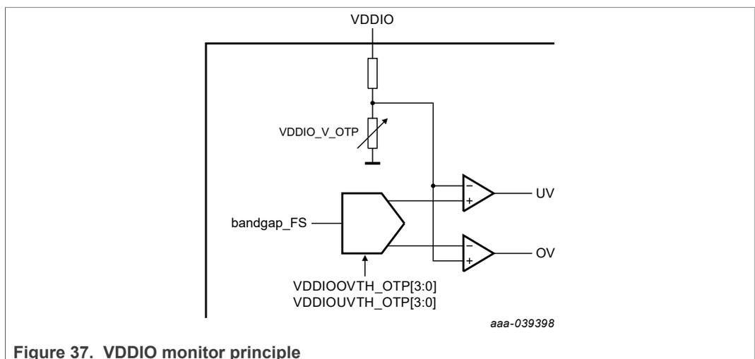
Figure 37. VDDIO monitor principle
