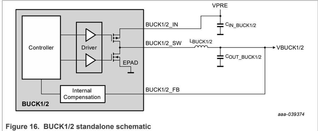
Figure 16. BUCK1/2 standalone schematic
