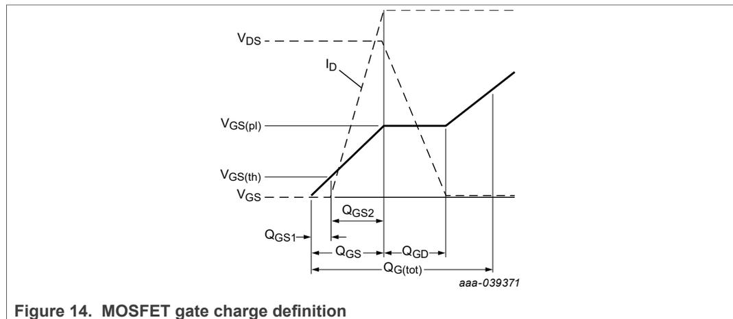
Figure 14. MOSFET gate charge definition
