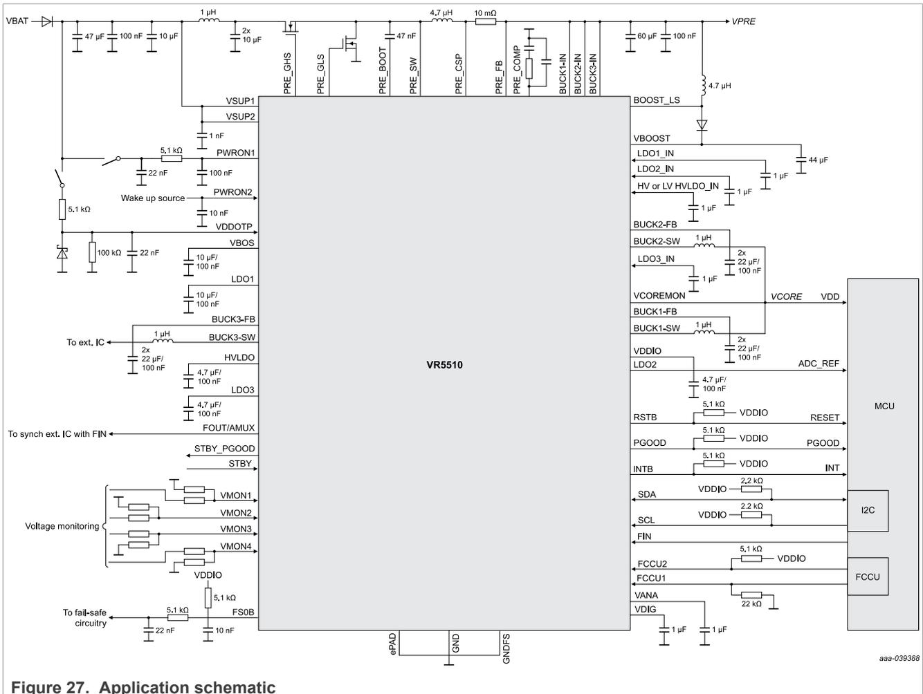
Figure 27. Application schematic
