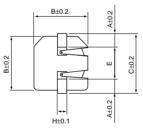
The lead terminal structure : The same bent lead type (refer to p.76) that is currently used on 10mm diameter and smaller parts, is also available upon request.
