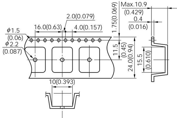
**Relay orientation mark and tape carrying direction.**
