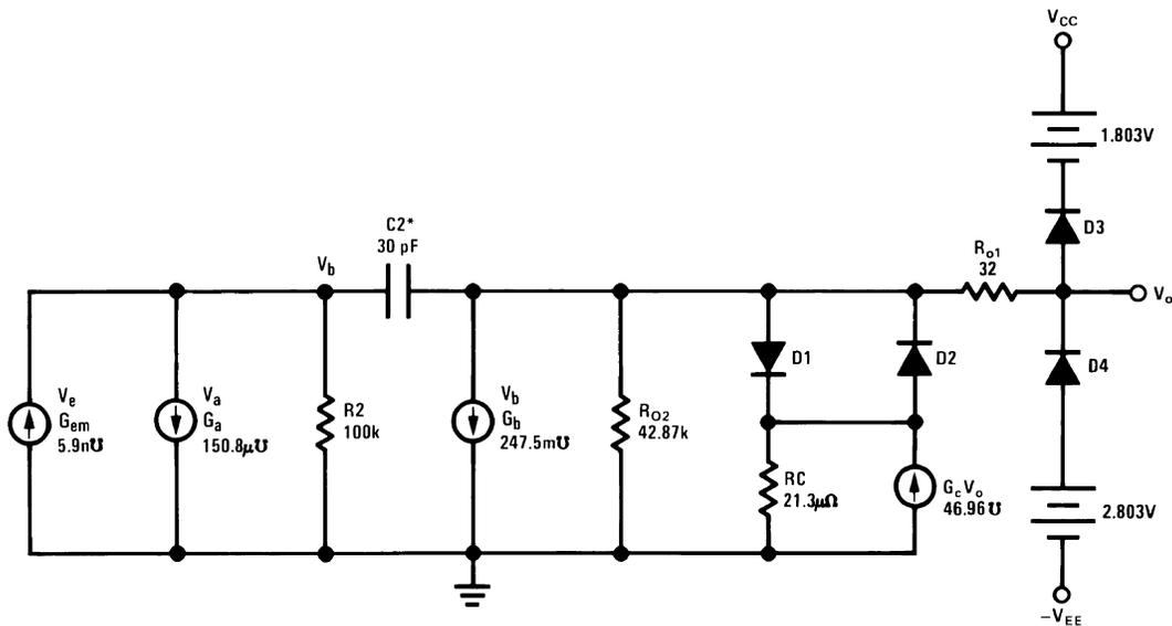
Figure 28. LM148, LM741 Macromodel for Computer Simulation
