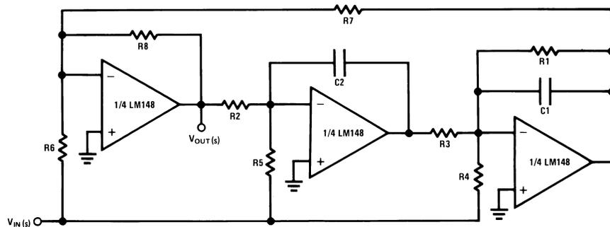
$$Q = \sqrt{\frac{R8}{R7}} \times \frac{R1C1}{\sqrt{R3C2R2C1}}, \quad f_o = \frac{1}{2\pi} \sqrt{\frac{R8}{R7}} \times \frac{1}{\sqrt{R2R3C1C2}}, \quad f_{NOTCH} = \frac{1}{2\pi} \sqrt{\frac{R6}{R3R5R7C1C2}}$$
