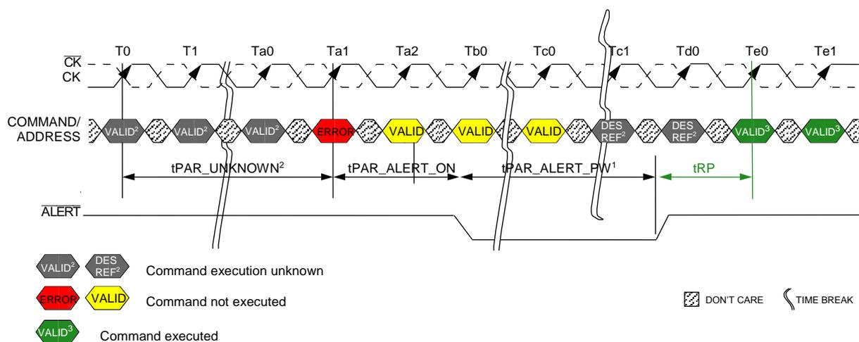
NOTE 1 DRAM is emptying queues. Precharge all and parity checking off until Parity Error Status bit cleared.
