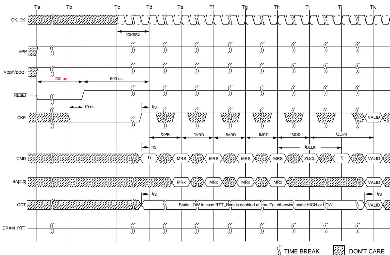
NOTE 1 From the time point  $T_d$  until  $T_k$ , a DES command must be applied between MRS and ZQCL commands.
