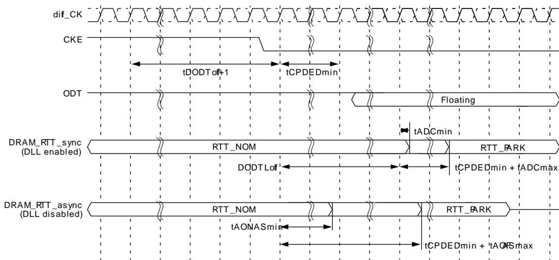
When exit from power down, along with CKE being registered high, ODT input signal must be re-driven and maintained low until  $t_{XP}$  is met.
