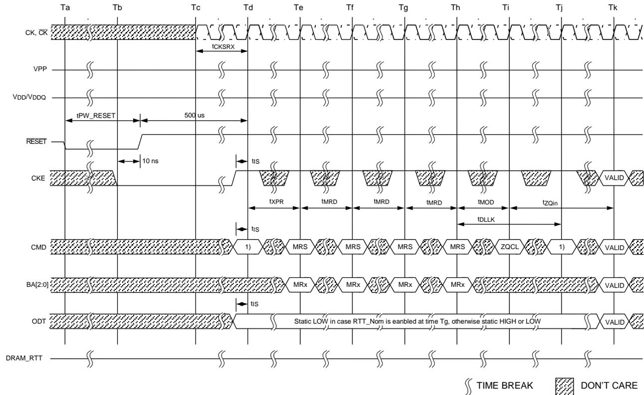
NOTE 1 From the time point Td until Tk, a DES command must be applied between MRS and ZQCL commands.
