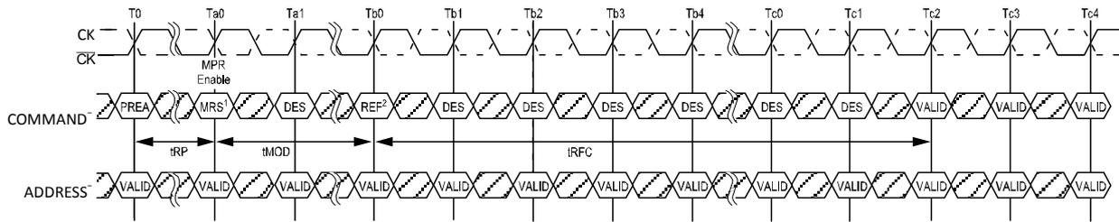
NOTE 1 Multipurpose registers Read/Write Enable (MR3 A2 = 1). Redirect all subsequent read and writes to MPR locations.
