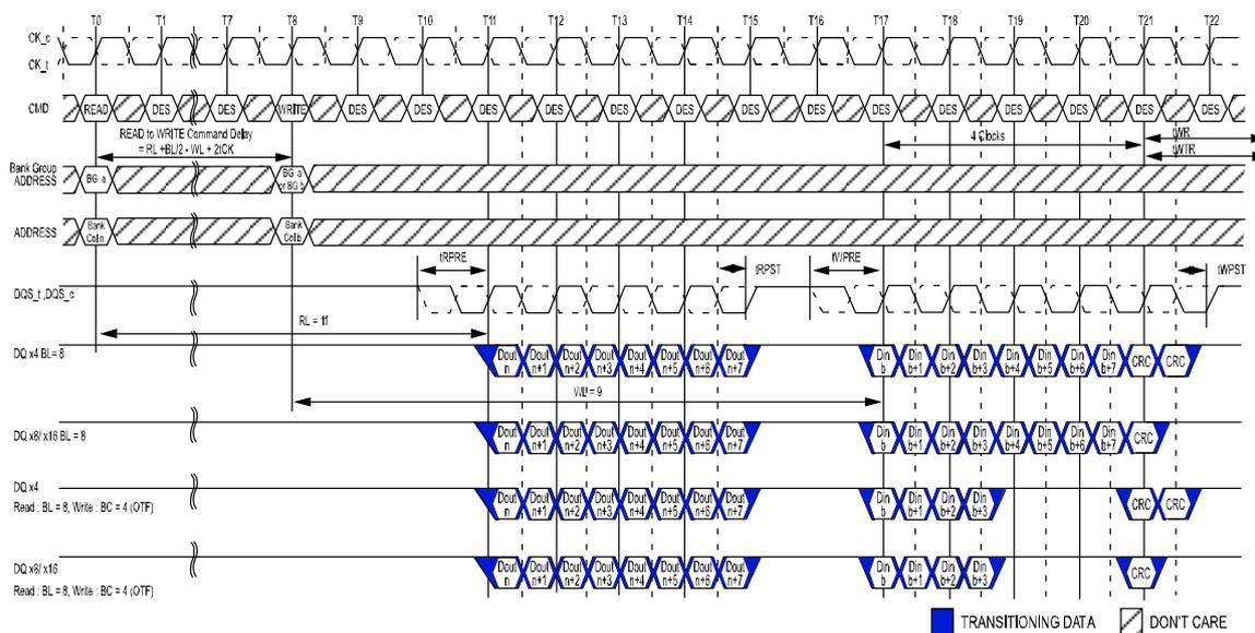
NOTE 1 BL = 8 (or BC = 4: OTF for Write), RL = 11 (CL = 11, AL = 0), Read Preamble = 1tCK, WL=9 (CWL=9, AL=0), Write Preamble = 1tCK
