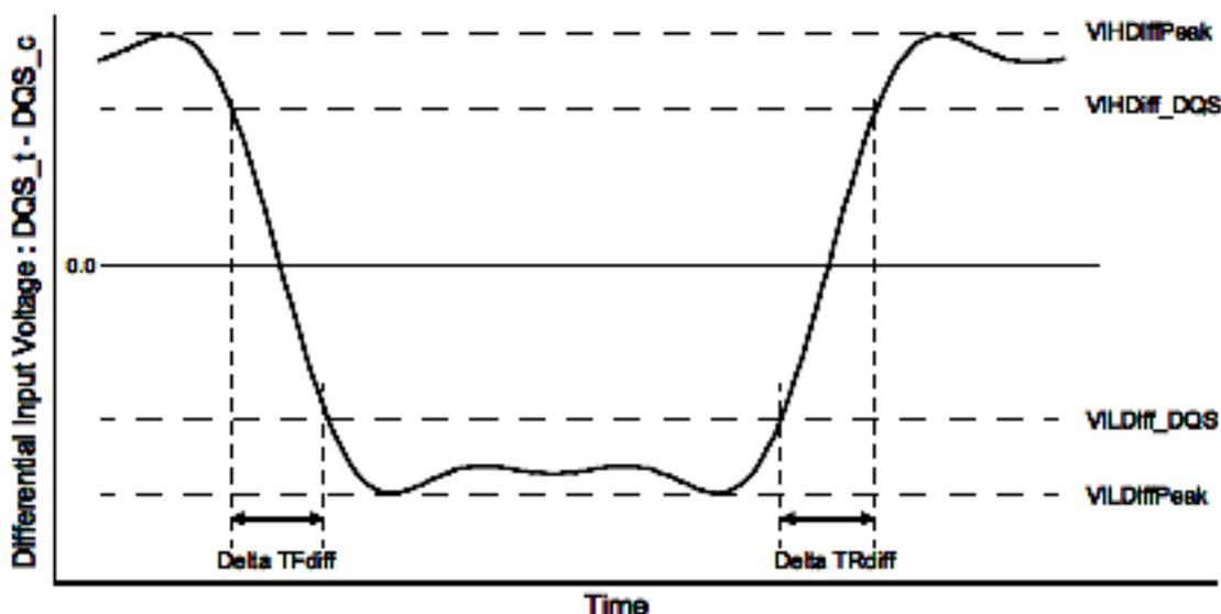
NOTE 1 Differential signal rising edge from VILDif\_DQS to VIHDiff\_DQS must be monotonic slope.
