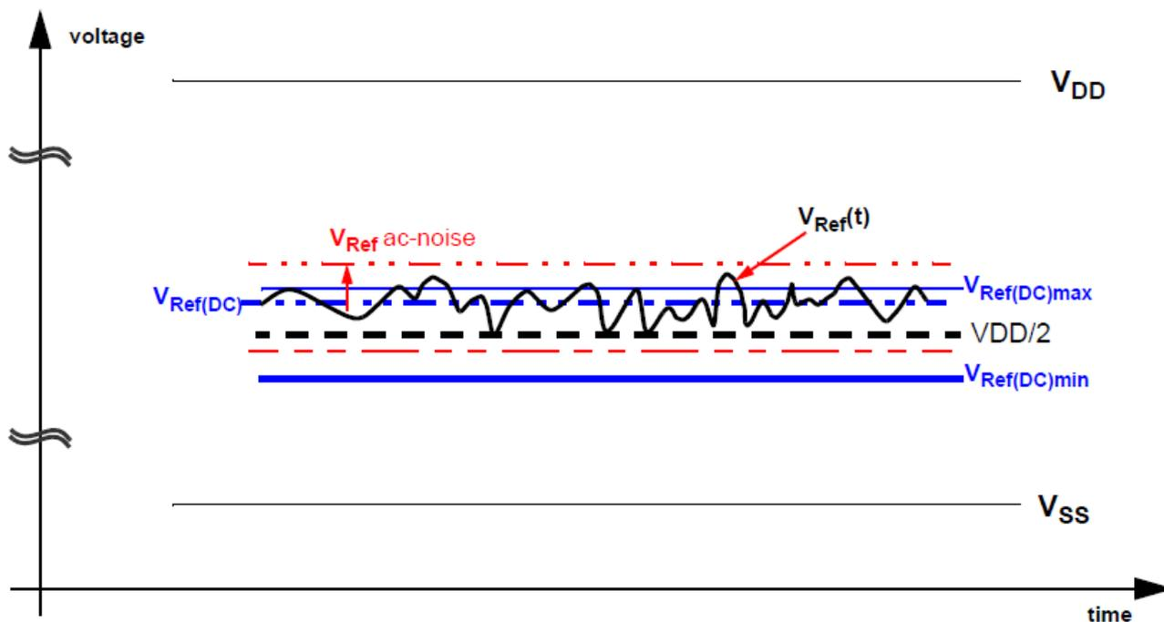
The voltage levels for setup and hold time measurements  $V_{IH}(AC)$ ,  $V_{IH}(DC)$ ,  $V_{IL}(AC)$  and  $V_{IL}(DC)$  are dependent on  $V_{REF}$ . "VREF" shall be understood as  $V_{REF}(DC)$ , as defined in Illustration of V.
