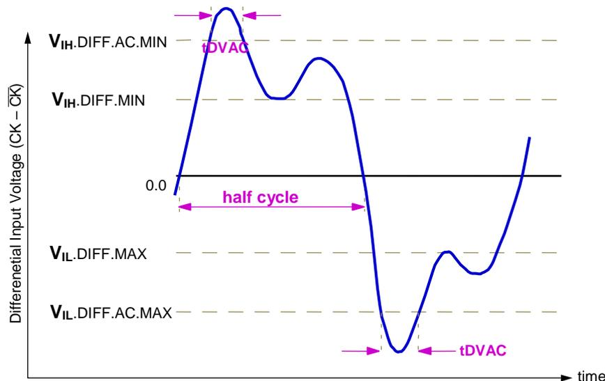
NOTE 1 Differential signal rising edge from  $V_{IL\_DIFF\_MAX}$  to  $V_{IH\_DIFF\_AC\_MIN}$  must be monotonic slope.
