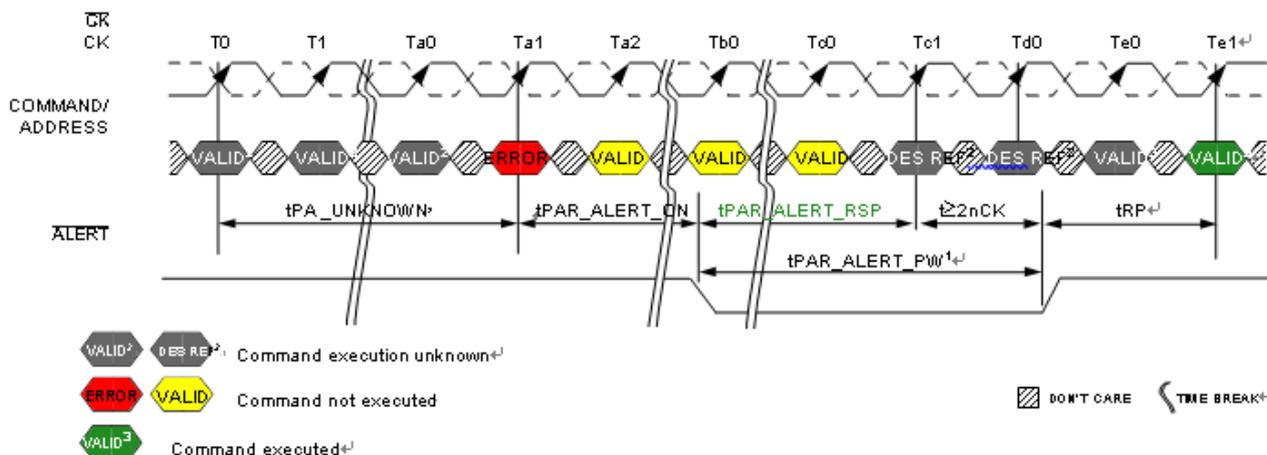
NOTE 1 DRAM is emptying queues. Precharge all and parity check re-enable finished by tPAR\_ALERT\_PW.
