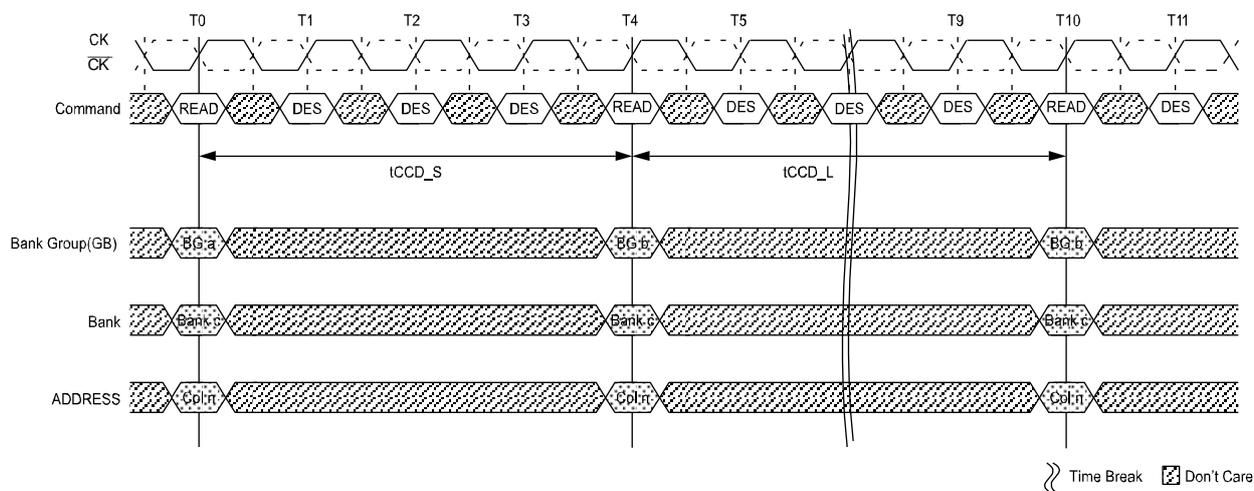
NOTE 1 tCCD\_S;  $\overline{\text{CAS}}$ -to- $\overline{\text{CAS}}$  delay (short). Applies to consecutive  $\overline{\text{CAS}}$  to different bank groups (i.e., T0 to T4).
