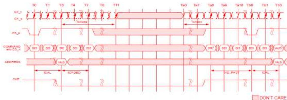
NOTE 1  $t_{CAL} = 3nCK$ ,  $t_{CPDED} = 4nCK$ ,  $t_{CKSRE} = 8nCK$ ,  $t_{CKSRX} = 8nCK$ ,  $t_{XS\_FAST} = t_{RFC4}(\min) + 10ns$
