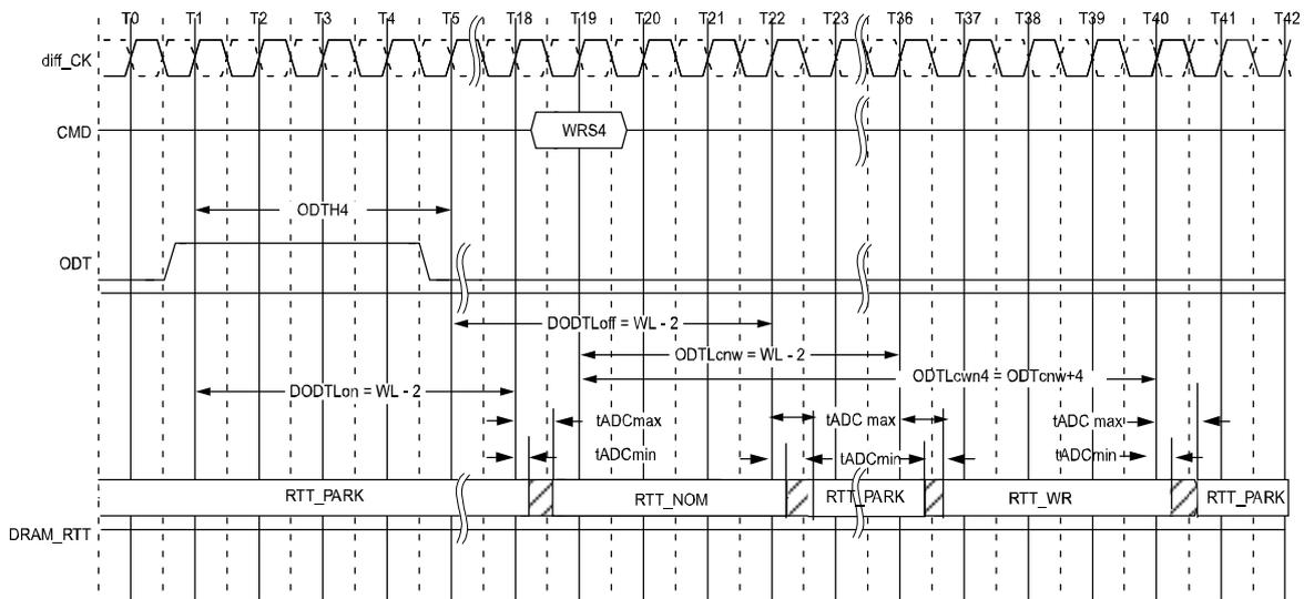
ODT must be held HIGH for at least ODT<sub>H4</sub> after assertion (T1). ODT<sub>H4</sub> is measured from ODT first registered HIGH to ODT first registered LOW, or from registration of Write command. Note that ODT<sub>H4</sub> should be adjusted depending on CRC or 2tCK preamble setting
