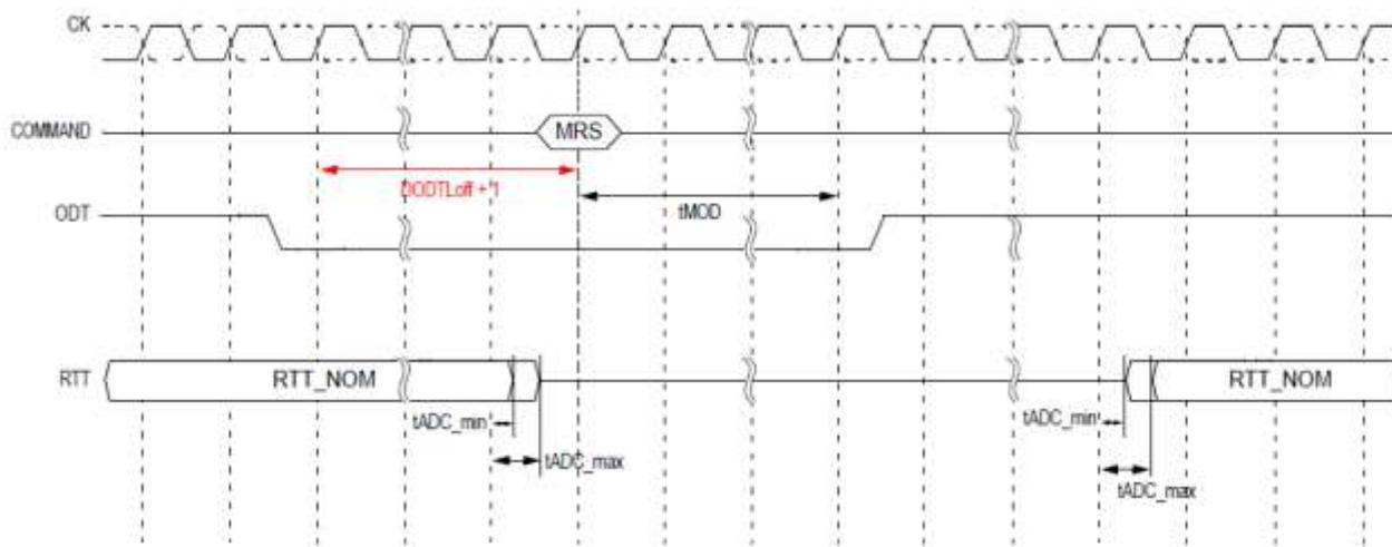
NOTE 1 This timing diagram shows CA Parity Latency mode is "Disable" case.
