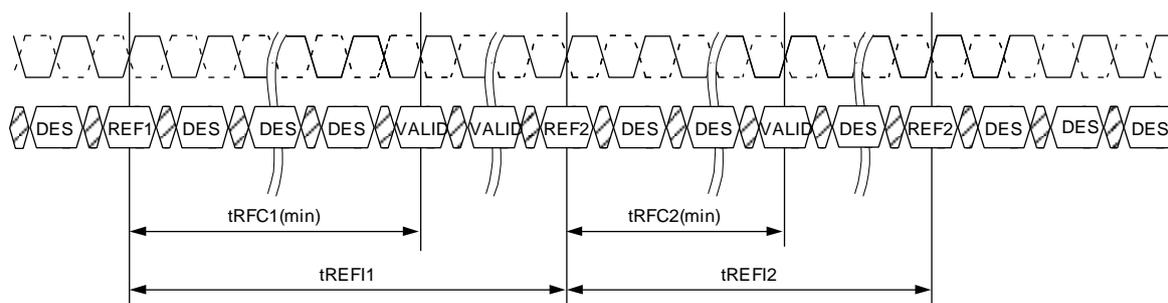
The following conditions must be satisfied before the refresh rate can be changed. Otherwise, data retention of DDR4 SDRAM cannot be guaranteed.
