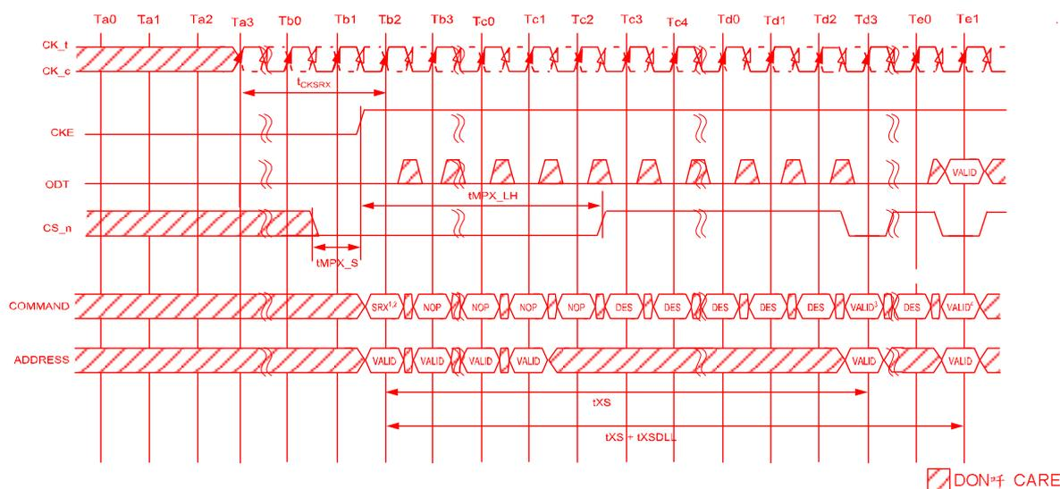
NOTE 1  $\overline{CS} = L, \overline{ACT} = H, \overline{RAS}/A16 = H, \overline{CAS}/A15 = H, \overline{WE}/A14 = H$  at Tb2 (No Operation command)
