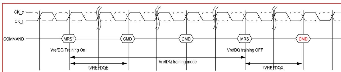
NOTE 1 The MR command used to enter VrefDQ Calibration Mode treats MR6 A [5:0] as don’t care while the next subsequent MR command sets VrefDQ values in MR6 A[5:0]
