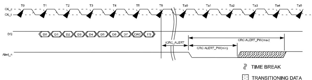
NOTE 1 CRC\_ALERT\_PW is specified from the point where the DRAM starts to drive the signal low to the point where the DRAM driver releases and the controller starts to pull the signal up.
