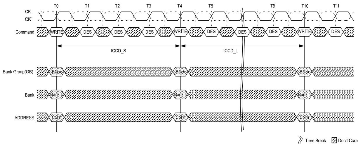
NOTE 1 tCCD\_S;  $\overline{\text{CAS}}$ -to- $\overline{\text{CAS}}$  delay (short). Applies to consecutive  $\overline{\text{CAS}}$  to different bank groups (i.e., T0 to T4).
