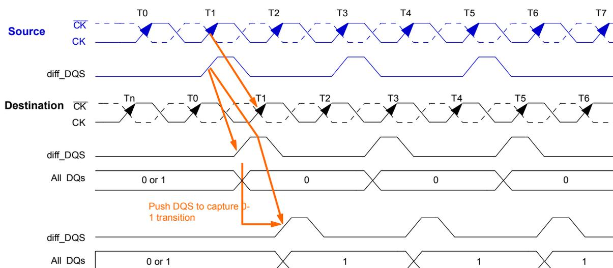
DQS -  $\overline{\text{DQS}}$  driven by the controller during leveling mode must be terminated by the DRAM based on the ranks populated. Similarly, the DQ bus driven by the DRAM must also be terminated at the controller.
