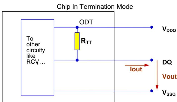
**ODT Electrical Characteristics RZQ=240Ω +/-1% entire temperature operation range after ZQ calibration**
