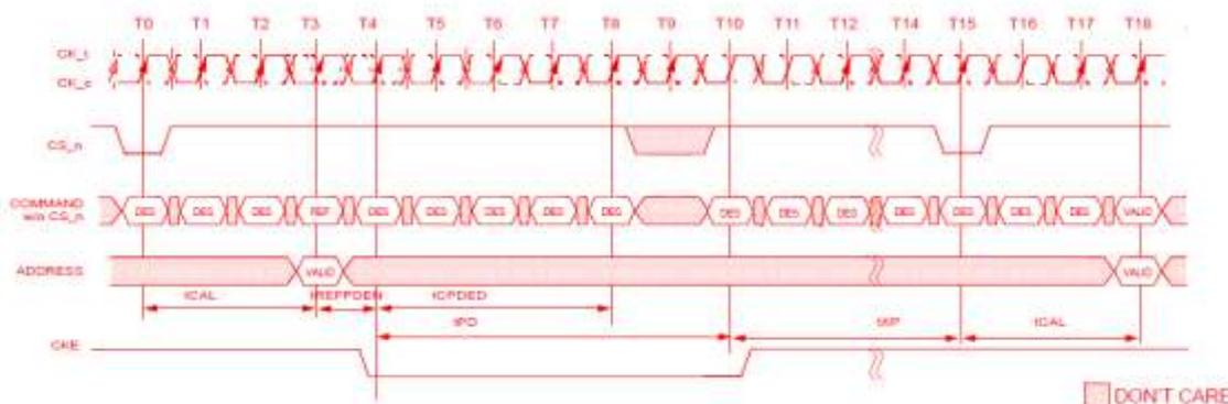
NOTE 1  $t_{CAL} = 3nCK$ ,  $t_{REFPDEN} = 1nCK$ ,  $t_{CPDED} = 4nCK$ ,  $t_{PD} = 6nCK$ ,  $t_{XP} = 5nCK$ .
