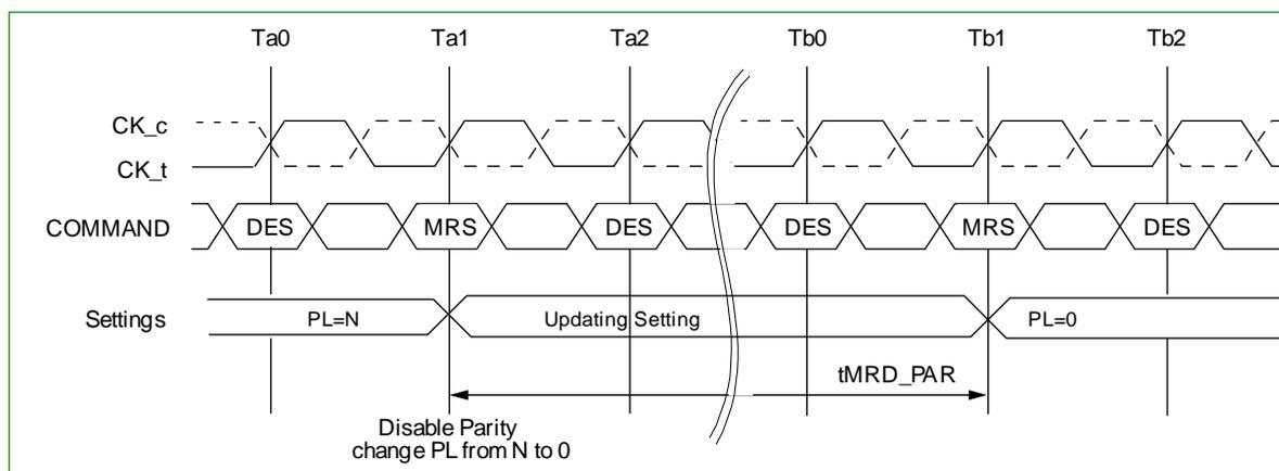
NOTE 1  $tMRD\_PAR = tMOD + N$ ; where N is the programmed parity latency prior to the MRS command exiting CA parity mode.
