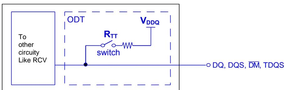
The switch is enabled by the internal ODT control logic, which uses the external ODT pin and Mode Register Setting and other control information. The value of  $R_{TT}$  is determined by the settings of mode register bits (see Mode Register). The ODT pin will be ignored if the mode register MR1 is programmed to disable  $R_{TT\_NOM}$  (MR1 A [10:8] = 000) and in self refresh mode.
