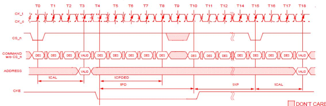
NOTE 1  $t_{CAL} = 3nCK$ ,  $t_{CPDED} = 4nCK$ ,  $t_{PD} = 6nCK$ ,  $t_{XP} = 5nCK$
