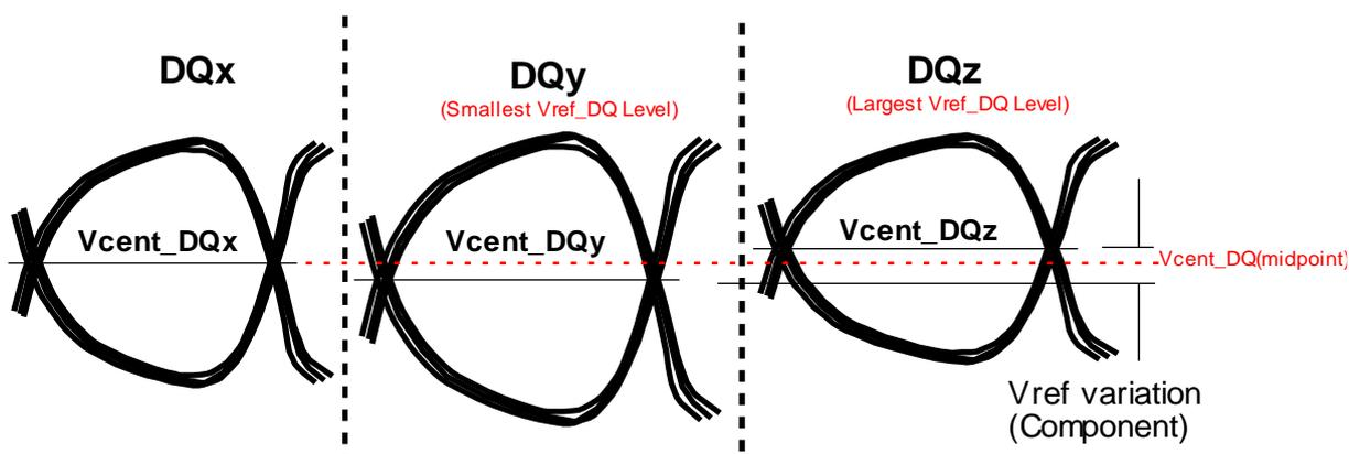
Vcent\_DQ(midpoint) is defined as the midpoint between the largest VREFDQ voltage level and the smallest VREFDQ voltage level across all DQ pins for a given DRAM. Each DQ pin's VREFDQ is defined by the center, i.e. widest opening, of the cumulative data input eye as depicted in below. This means a DRAM's level variation is accounted for within the DRAM Rx mask. The DRAM VREFDQ level will be set by the system to account for Ron and ODT settings.
