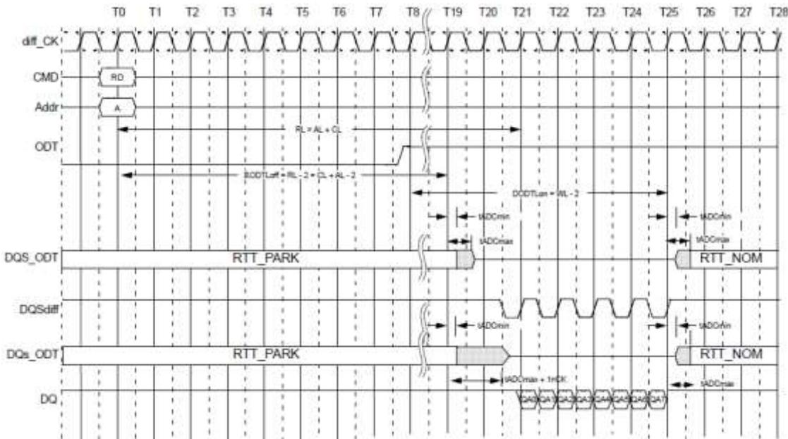
**Example: CL=11, PL=0; AL=CL-1=10; RL=AL+PL+CL=21; CWL=9; DODTLon= AL+CWL-2=17; DODTLoff=AL+CWL-2=17; 2tCK preamble)**
