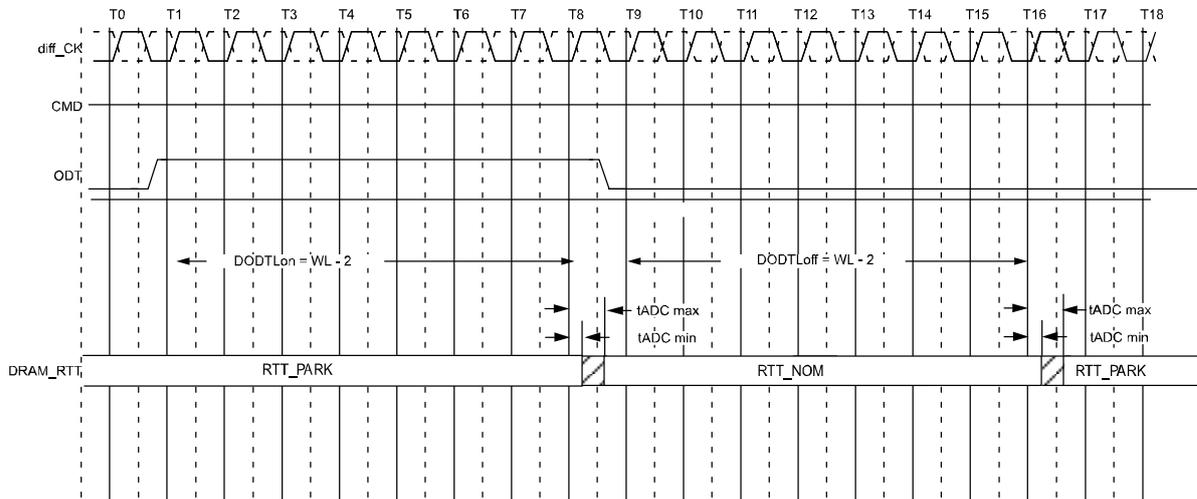
**Synchronous ODT example with BL=4, CWL=9, AL=10, PL=0; DODTLon/off=WL-2=17,
