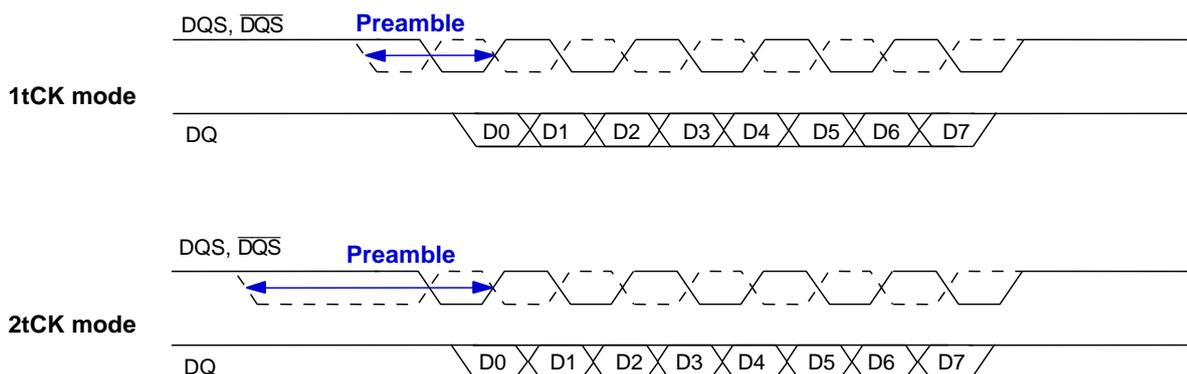
When operating in 2 tCK Write preamble mode in MR2 CWL (CAS Write Latency), CWL of 1st Set needs to be incremented by 2 nCK and CWL of 2nd Set does not need increment of it. tWTR must be increased by one clock cycle from the tWTR required in the applicable speed bin table. WR must be programmed to a value one or two clock cycle(s), depending on available settings, greater than the WR setting required per the applicable speed bin table.
