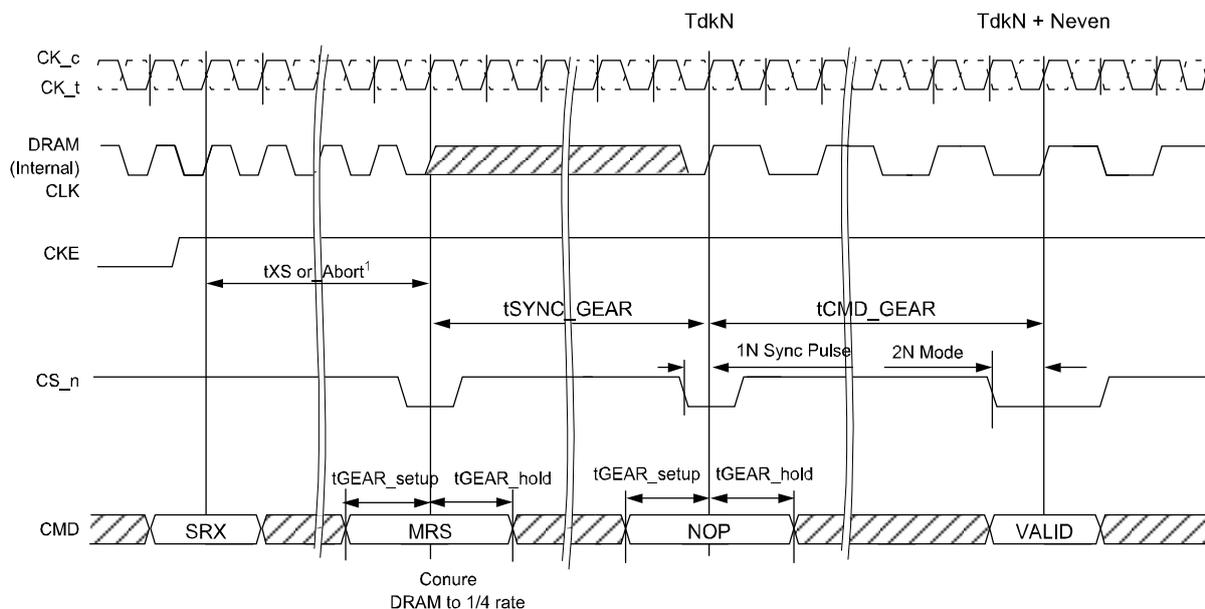
NOTE 1 CKE High Assert to Gear Down Enable Time ( $t_{XS}$ ,  $t_{XS\_Abort}$ ) depend on MR setting. A correspondence of  $t_{XS}/t_{XS\_Abort}$  and MR Setting is as follows. - MR4[A9] = 0:  $t_{XS}$  - MR4[A9] = 1:  $t_{XS\_Abort}$
