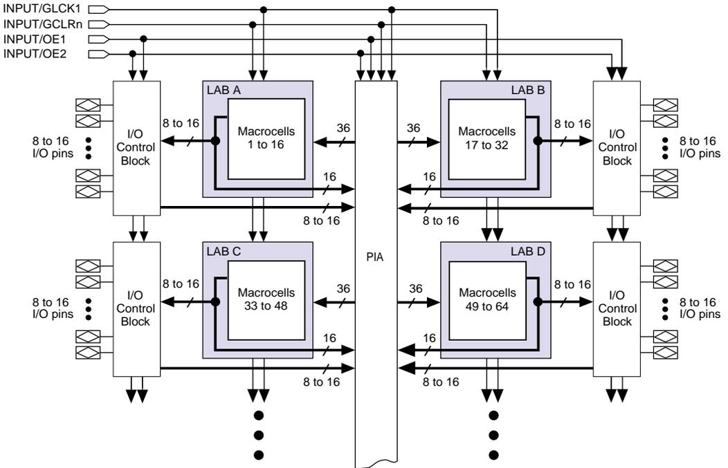
Figure 2 shows the architecture of MAX 7000E and MAX 7000S devices.
