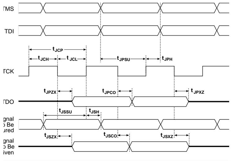
Table 9 shows the JTAG timing parameters and values for MAX 7000S devices.
