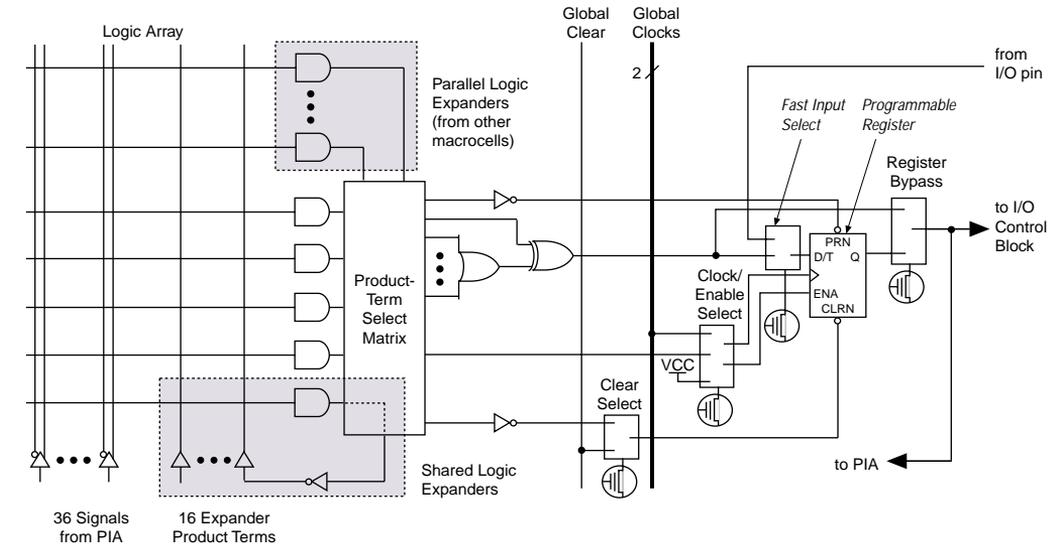
Combinatorial logic is implemented in the logic array, which provides five product terms per macrocell. The product-term select matrix allocates these product terms for use as either primary logic inputs (to the OR and XOR gates) to implement combinatorial functions, or as secondary inputs to the macrocell’s register clear, preset, clock, and clock enable control functions. Two kinds of expander product terms (“expanders”) are available to supplement macrocell logic resources:
