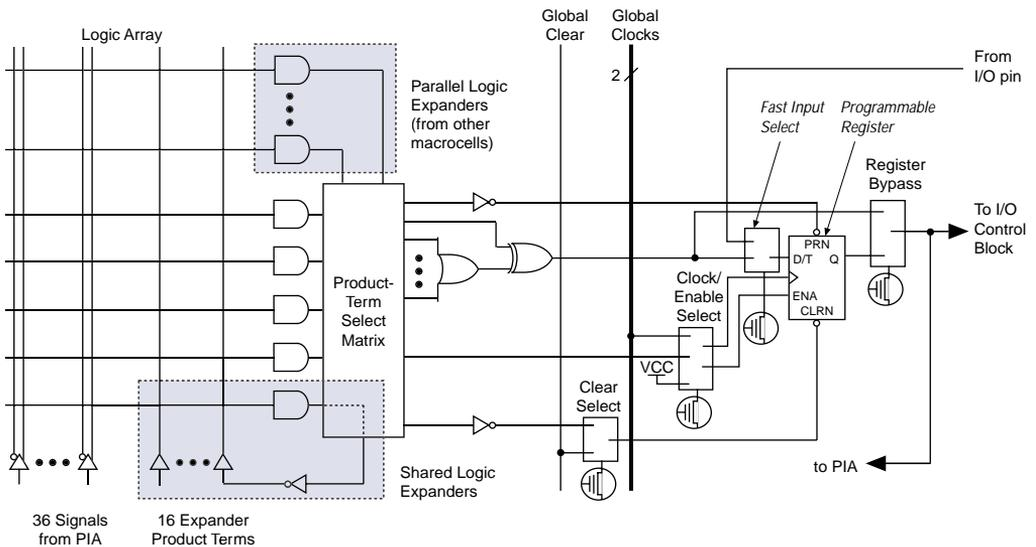
Figure 4 shows a MAX 7000E and MAX 7000S device macrocell.
