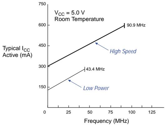
Figure 15 shows typical supply current versus frequency for MAX 7000S devices.
