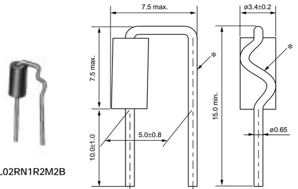
\*There is excess bond stick on the wire. (in mm)
