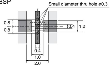
The chip EMI filter suppress noise by passing the high-frequency noise to ground. Therefore, to get noise suppression effectively, it is recommended to put through holes (ø0.3 mm) into the center and both sides of ground-pattern to connect to ground-plane.
