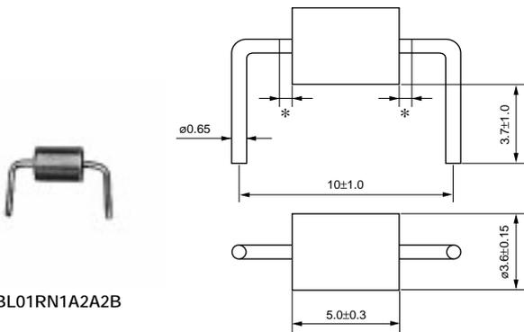
\*Coating extending on leads : 1.5 max. (in mm)
