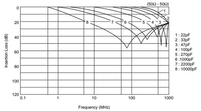
**Built-in Ferrite Beads DSS6 Series Incrimp Type**
