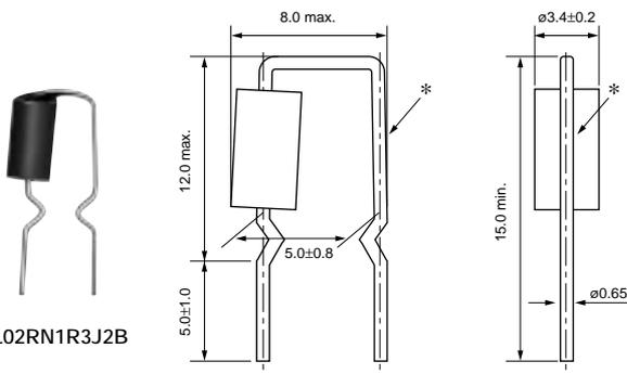
\*There is excess bond stick on the wire. (in mm)
