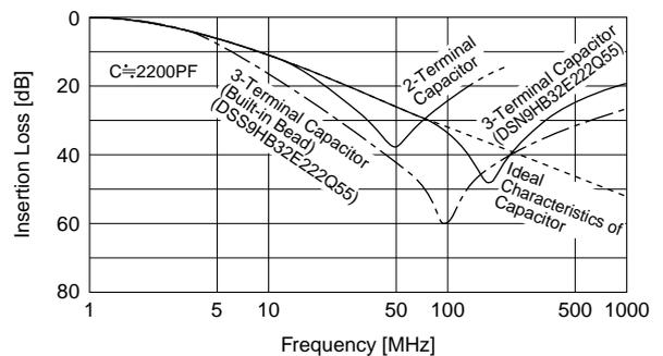
A 3-terminal capacitor has a higher self resonance frequency than a general 2-terminal type and exhibits effective noise suppression at high frequency.
