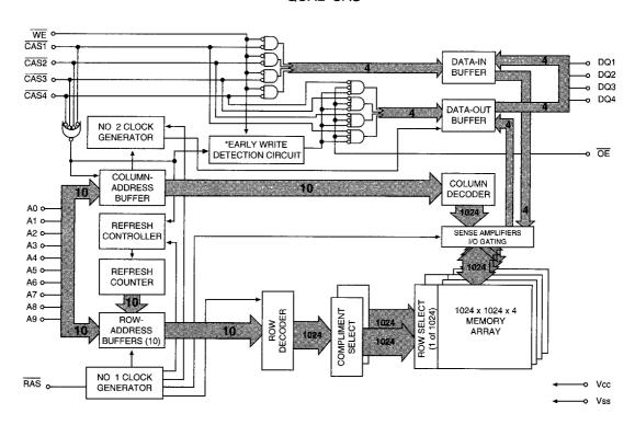
\*NOTE: 1. WE LOW prior to first CAS LOW, EW detection circuit output is a 1.
