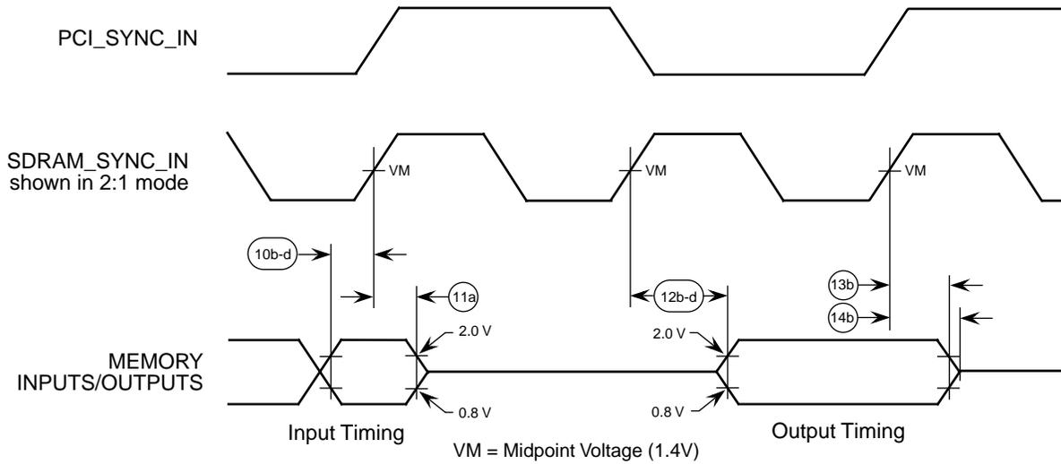
Figure 7. Input - Output Timing Diagram Referenced to SDRAM\_SYNC\_IN
