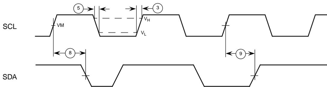
Figure 13. I<sup>2</sup>C Timing Diagram II
