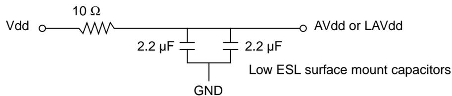
Figure 23. PLL Power Supply Filter Circuit
