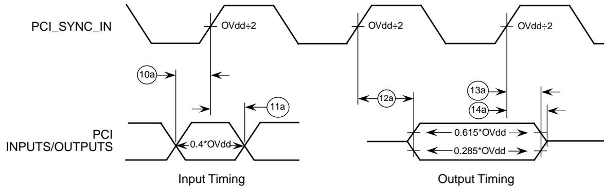
Figure 8. Input - Output Timing Diagram Referenced to PCI\_SYNC\_IN
