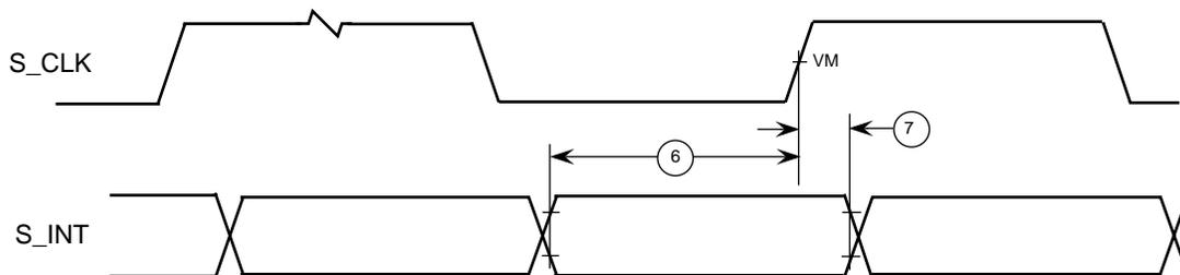
**Figure 17. PIC Serial Interrupt Mode Input Timing Diagram**
