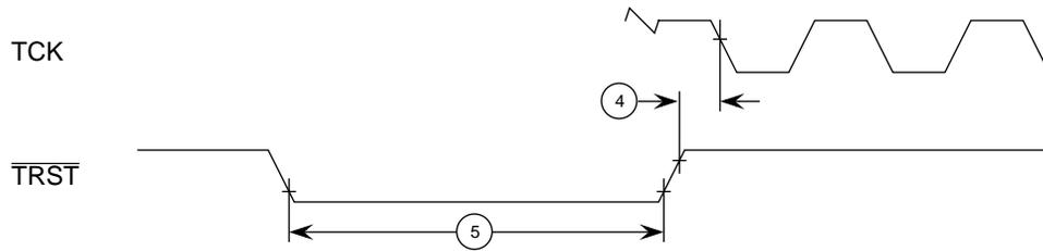
Figure 19. JTAG TRST Timing Diagram
