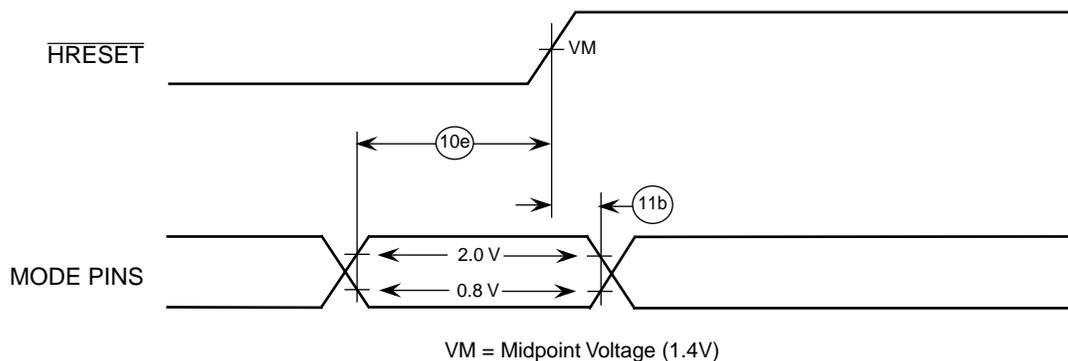
Figure 9. Input Timing Diagram for Mode Select Signals
