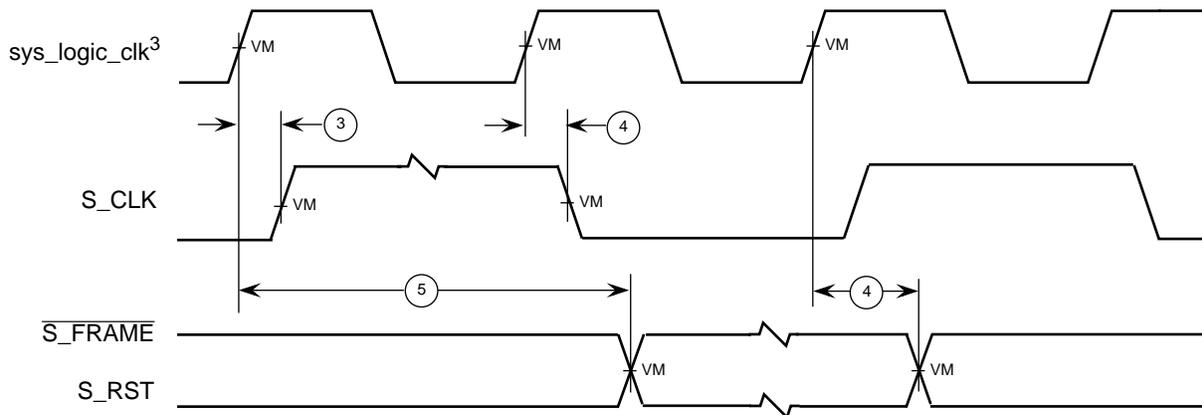
**Figure 16. PIC Serial Interrupt Mode Output Timing Diagram**
