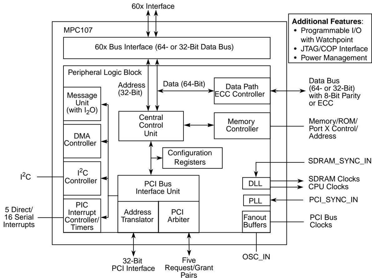
Figure 1. MPC107 Block Diagram
