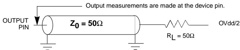
**Figure 10. AC Test Load for the MPC107**
