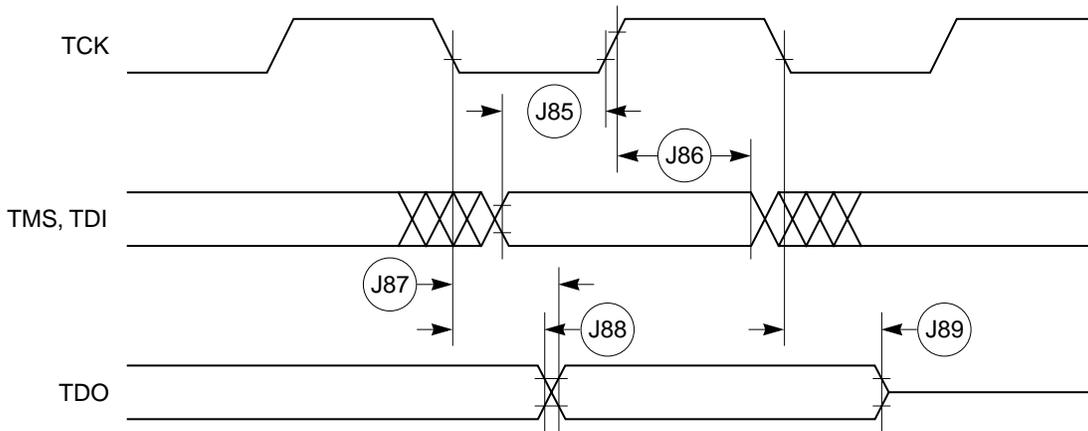
Figure 35. JTAG Test Access Port Timing Diagram
