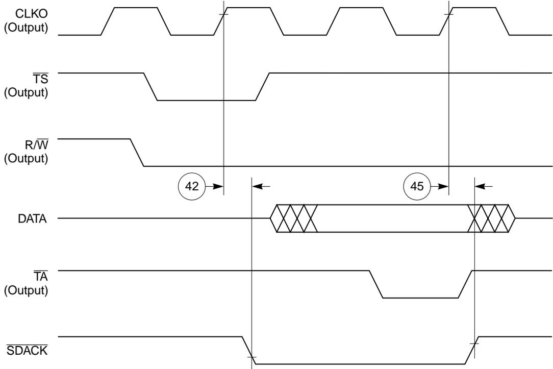
Figure 47.  $\overline{SDACK}$  Timing Diagram—Peripheral Read, Internally-Generated  $\overline{TA}$
