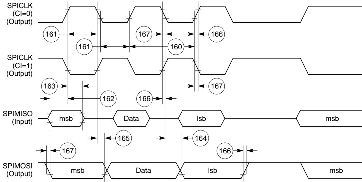
**Figure 64. SPI Master (CP = 0) Timing Diagram**
