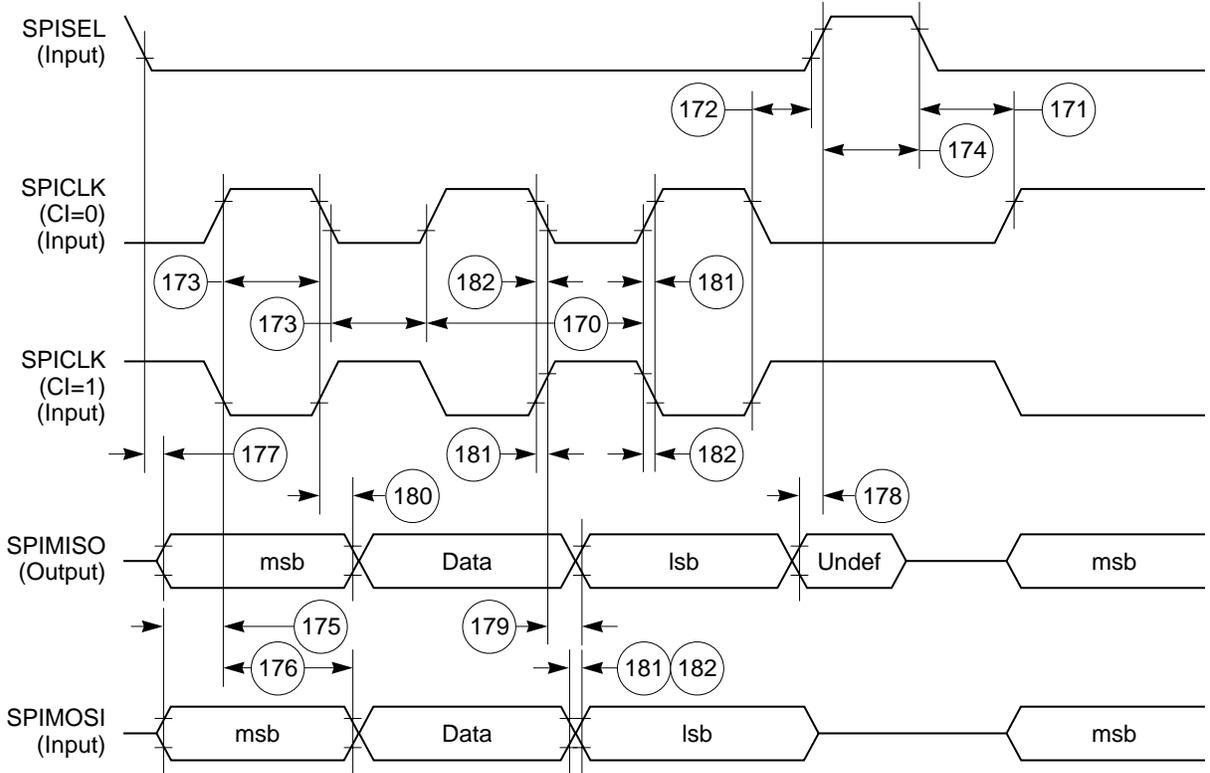
Figure 66. SPI Slave (CP = 0) Timing Diagram
