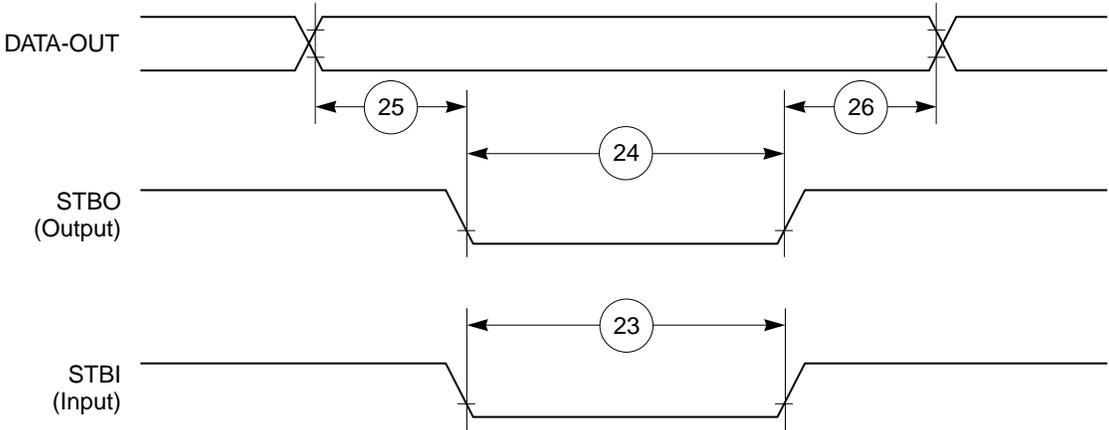
Figure 41. PIP TX (Pulse Mode) Timing Diagram
