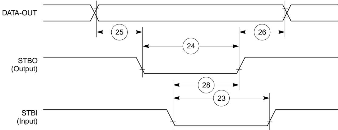
Figure 39. PIP Tx (Interlock Mode) Timing Diagram
