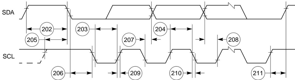
**Figure 68. I<sup>2</sup>C Bus Timing Diagram**
