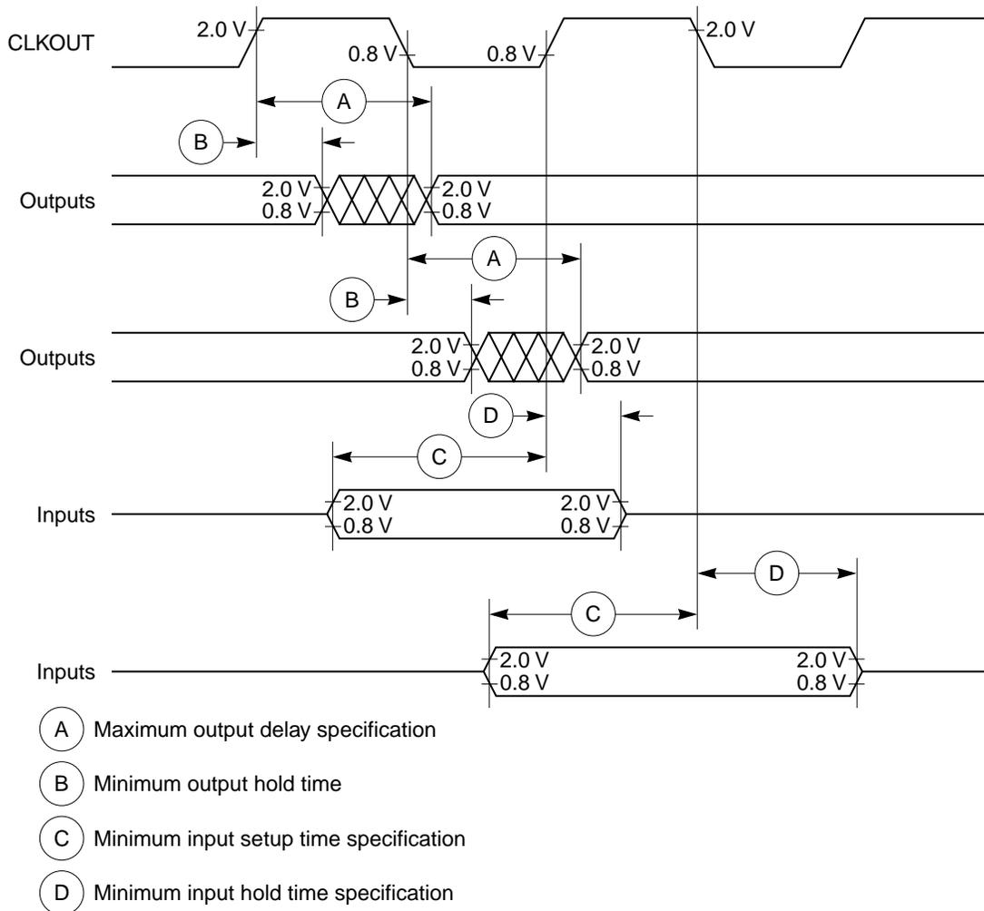
**Figure 2. Control Timing**
