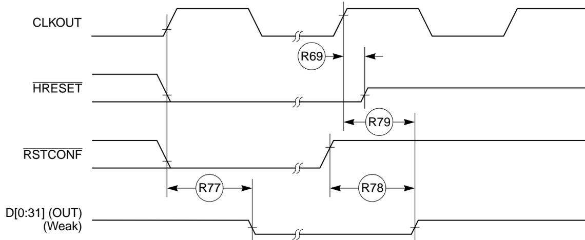
**Figure 32. Reset Timing—Data Bus Weak Drive During Configuration**
