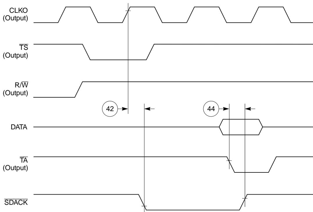
**Figure 46.  $\overline{SDACK}$  Timing Diagram—Peripheral Write, Internally-Generated  $\overline{TA}$**
