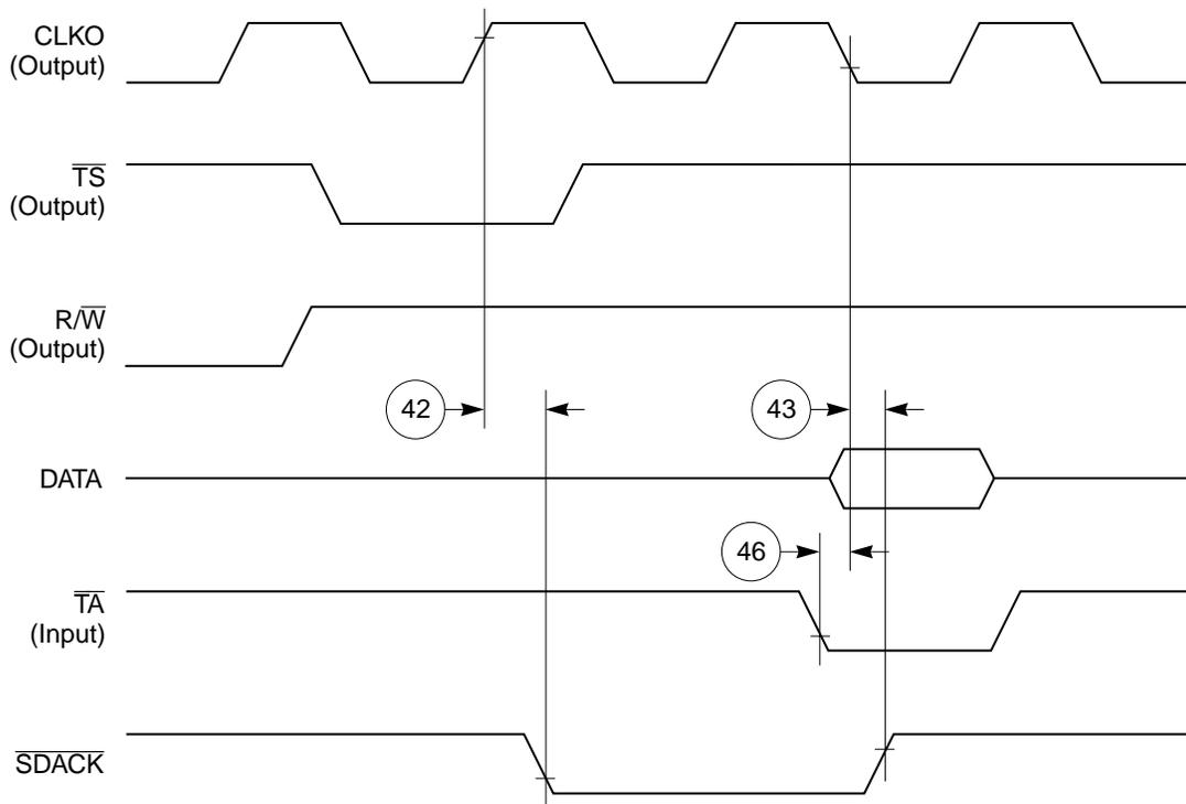
**Figure 45.  $\overline{SDACK}$  Timing Diagram—Peripheral Write, Externally-Generated  $\overline{TA}$**
