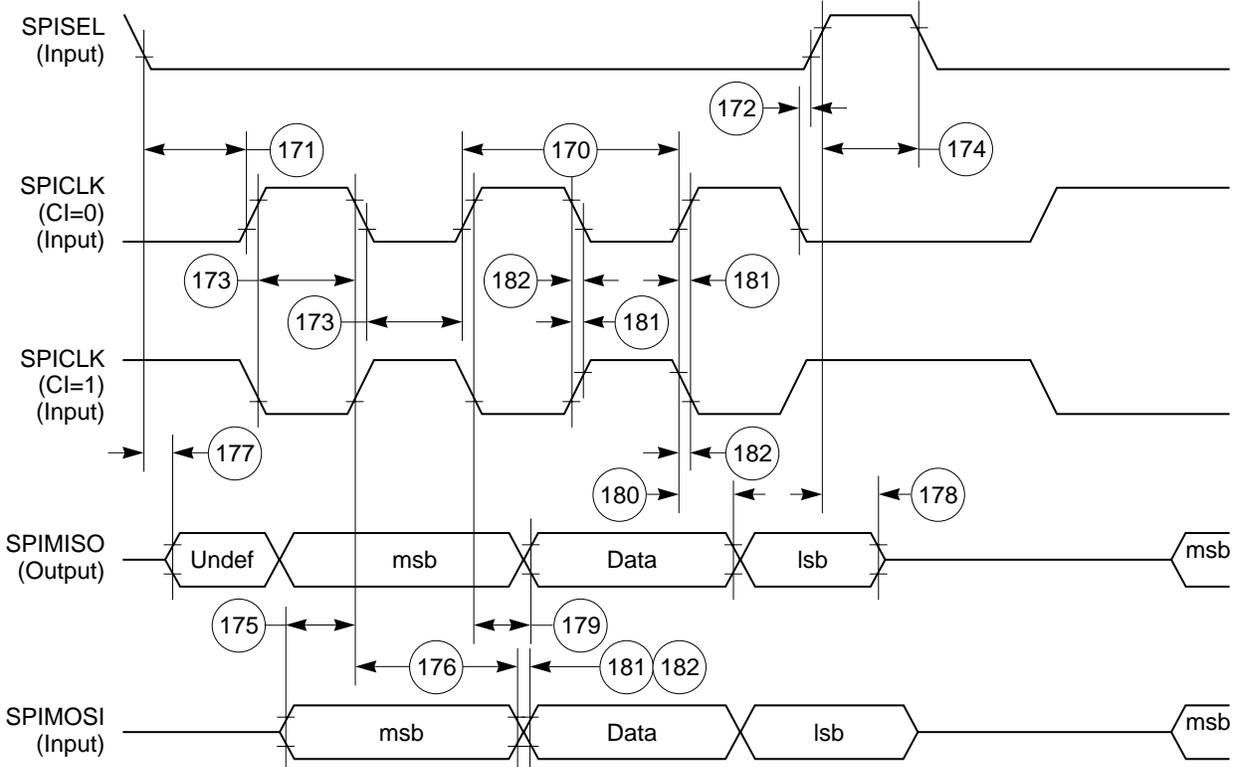
Figure 67. SPI Slave (CP = 1) Timing Diagram
