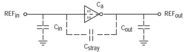
**Figure 20. Parasitic Capacitances of the Amplifier and C<sub>stray</sub>**
