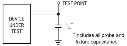
Figure 12. Test Circuit
