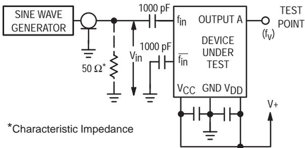
Figure 7. Test Circuit
