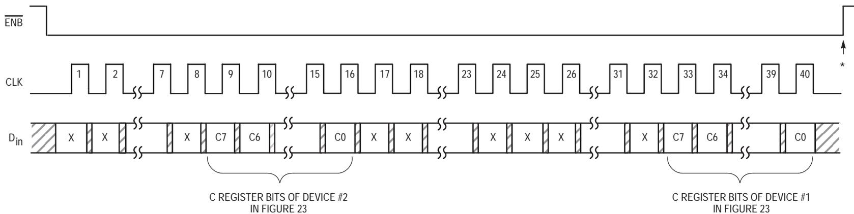
\*At this point, the new bytes are transferred to the C registers of both devices and stored. No other registers are affected.
