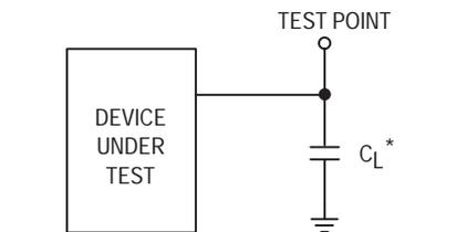
\*Includes all probe and fixture capacitance.
