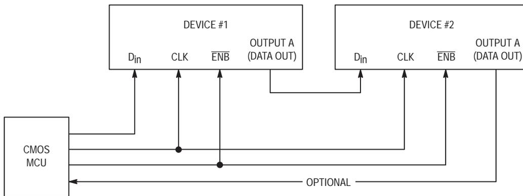
NOTE: See related Figures 24 through 26; these bit streams apply to the MC145190, MC145191, MC145200, and MC145201.
