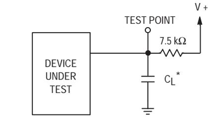
\*Includes all probe and fixture capacitance.
