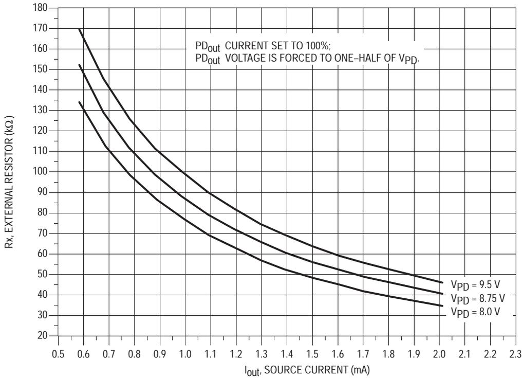
Nominal MC145190 PD<sub>out</sub> Source Current vs Rx Resistance
