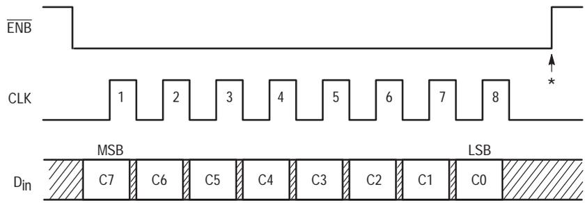
\* At this point, the new byte is transferred to the C register and stored. No other registers are affected.
