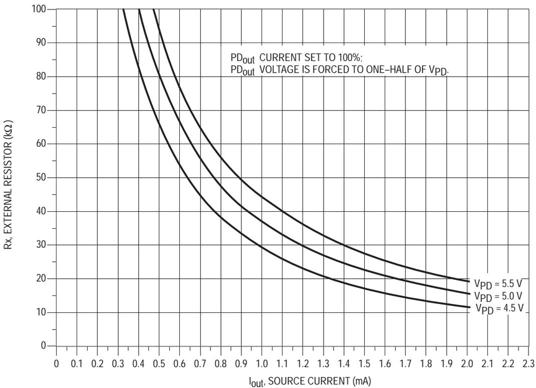
Nominal MC145191 PD<sub>out</sub> Source Current vs Rx Resistance
