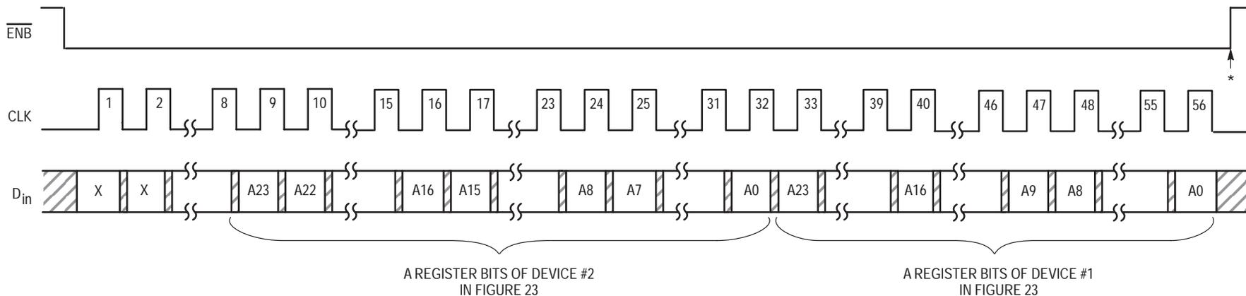
\*At this point, the new bytes are transferred to the A registers of both devices and stored. Additionally, for both devices, the 13 LSBs in each of the first buffers of the R registers are transferred to the respective R register's second buffer. Thus, the R, N, and A counters can be presented new divide ratios at the same time. The first buffer of each R register is not affected. Neither C register is affected.
