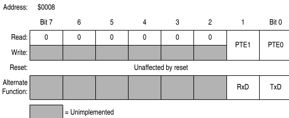
Figure 16-17. Port E Data Register (PTE)
