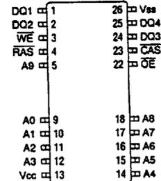
results in a READ WRITE cycle. The four data inputs and four data outputs are routed through four pins using common I/O and pin direction is controlled by WE and OE.
