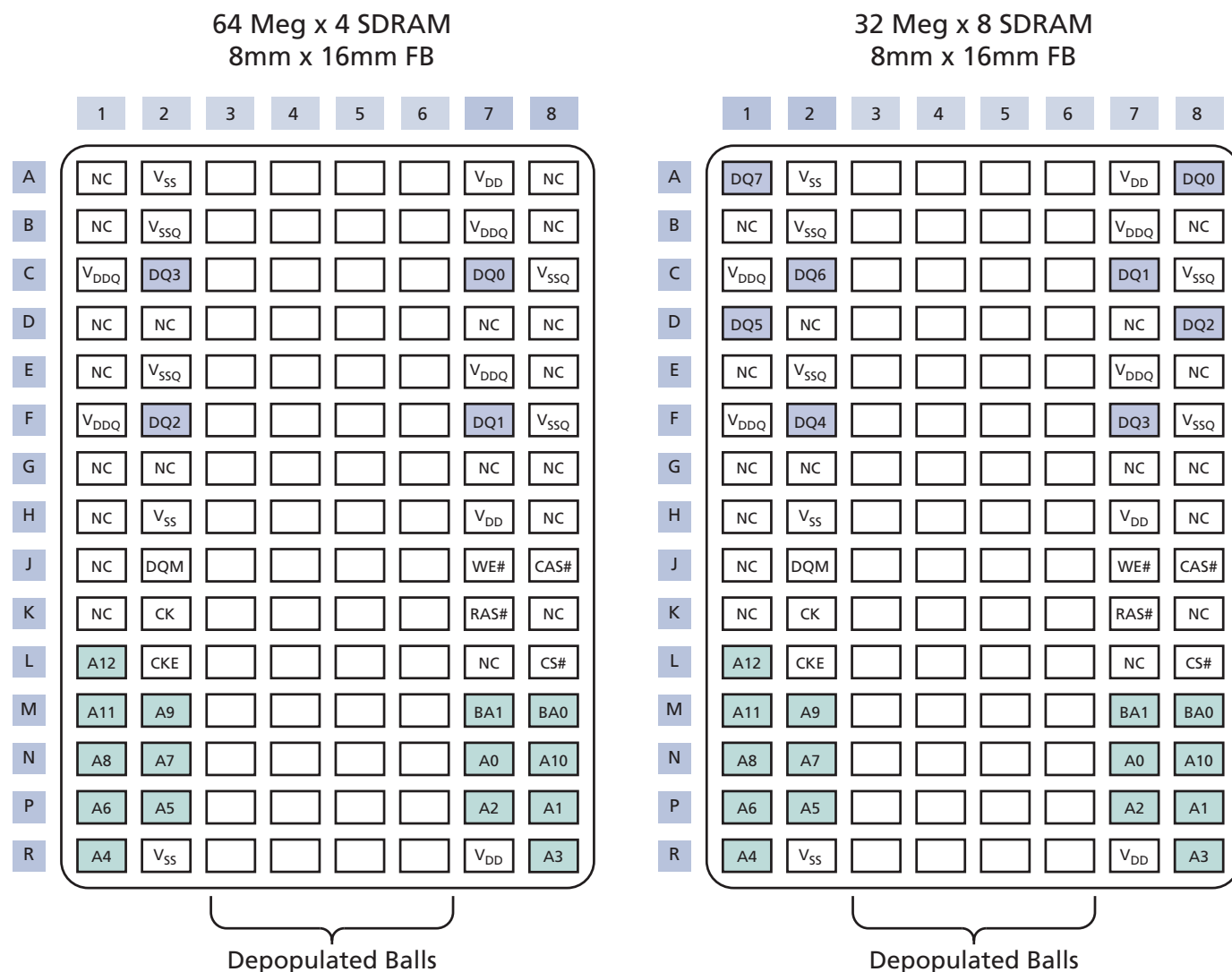
Figure 5: 60-Ball FBGA (Top View)
