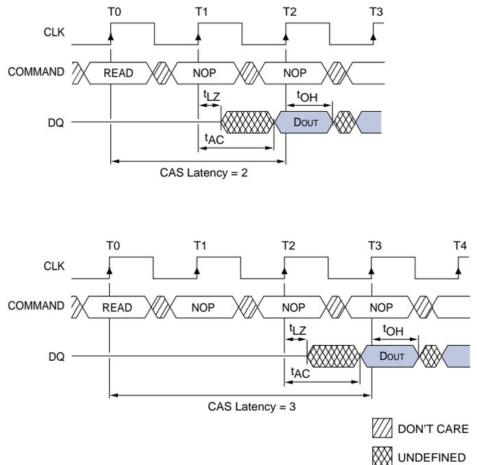
This is shown in Figure 7 for CAS latencies of two and three; data element  $n+3$  is either the last of a burst of four or the last desired of a longer burst. The 128Mb SDRAM uses a pipelined architecture and therefore does not require the  $2n$  rule associated with a prefetch architec-
