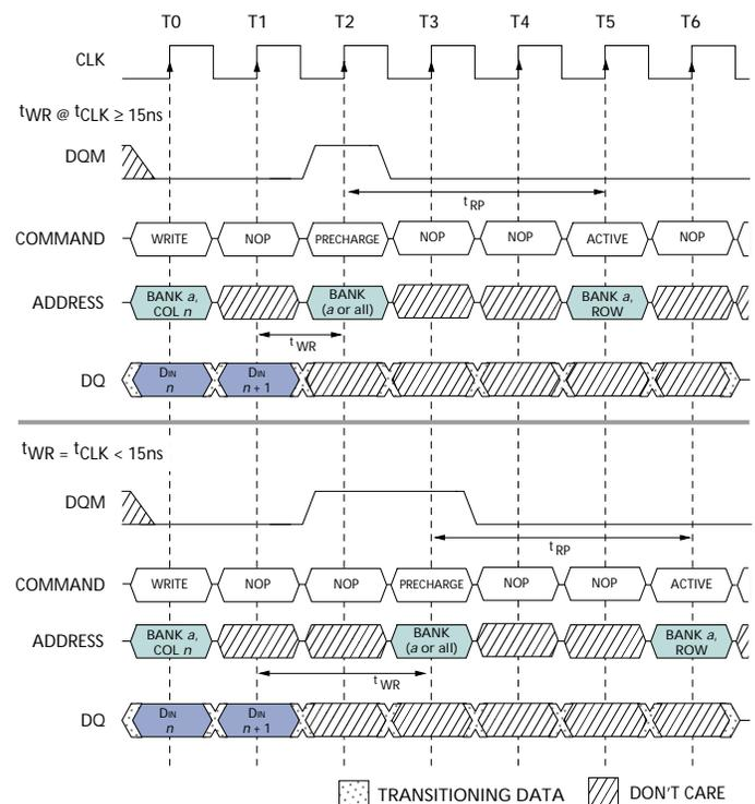
NOTE: DQM could remain LOW in this example if the WRITE burst is a fixed length of two.
